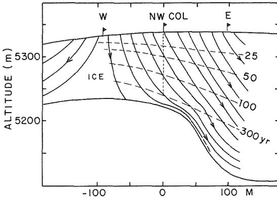
FIG. 3 Vertical cross section through the Northwest Col showing flow lines and time lines. Borehole is at central flag (Northwest Col).
