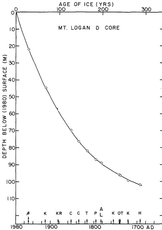
FIG. 2 Depth vs time scale plot for the Mt. Logan core. Volcanic events identified through the chemical signatures are marked by vertical arrows. The double arrow marks the end of the  $\beta$ -activity dating.
