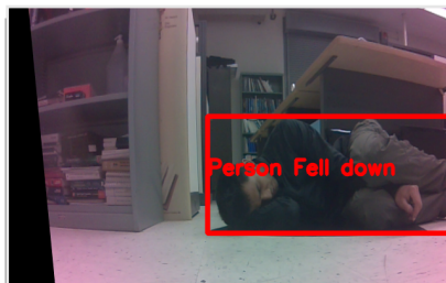
Figure 4.6: Top: Fall event detection in the presence of multiple people. Bottom: Fall detected by the robot, and sample email generated by the system.
