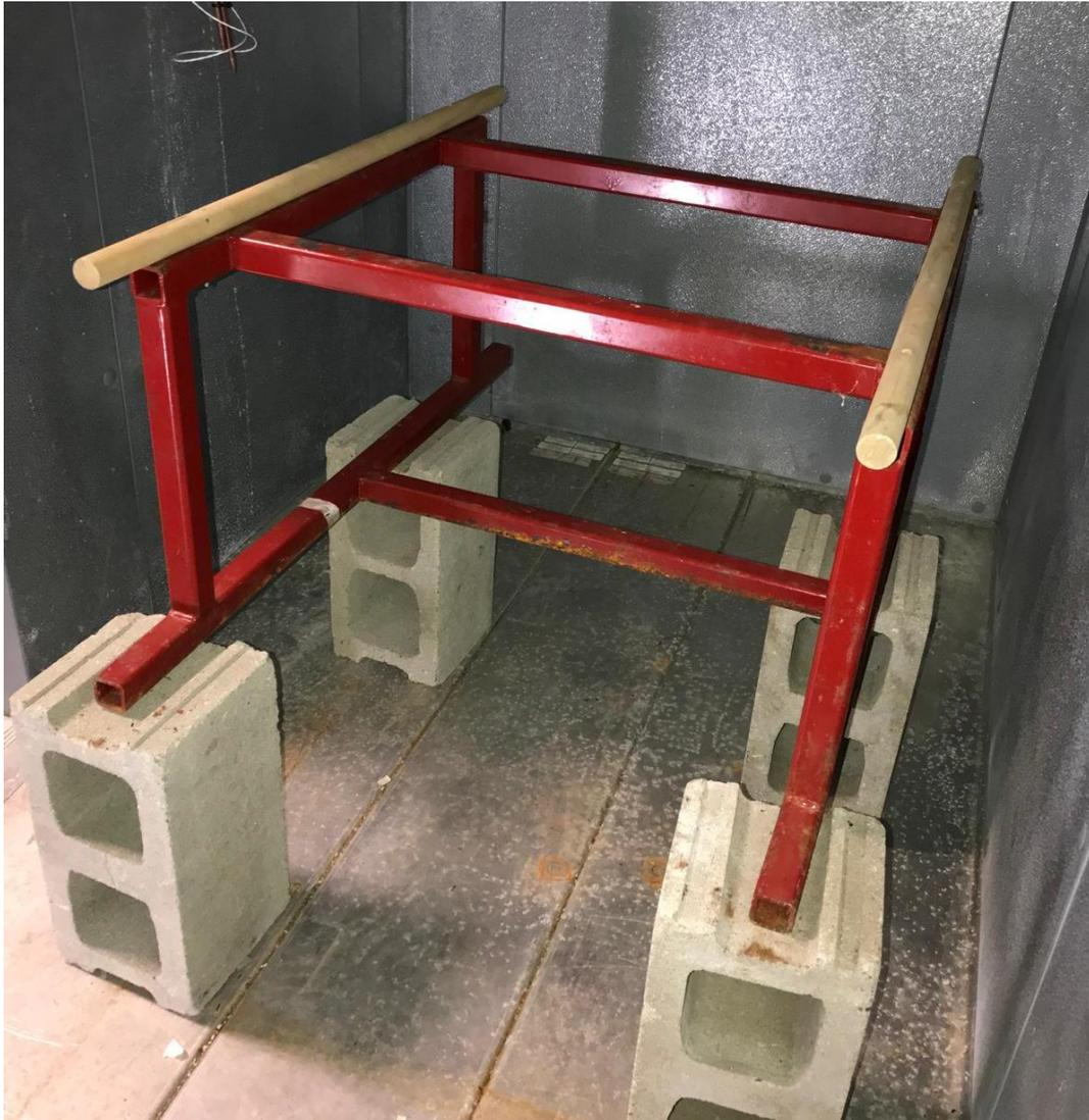
Figure 2. 5 Creep testing frame
