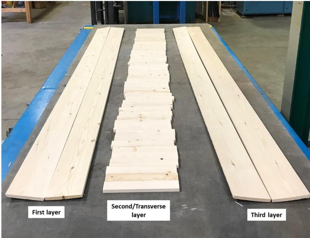
Figure 1. 1 Lumber boards laid side by side for CLT assembly
