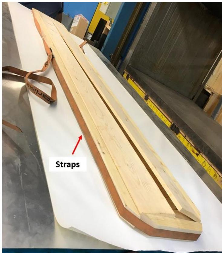
Figure 1. 2 CLT assembly before pressing
