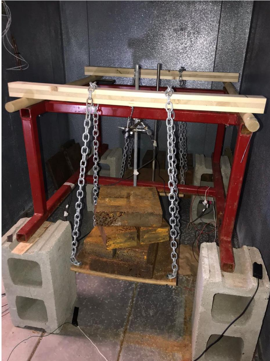
Figure 2. 6 Experimental creep test setup
