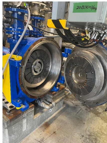
Figure 2.3: Dual-Disc CNF Refiner at the University of Maine Process Development Center (PDC).
