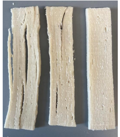
Figure 6.4: 6-cycle samples with observed expansion (left, middle) and 2-cycle sample (right).
