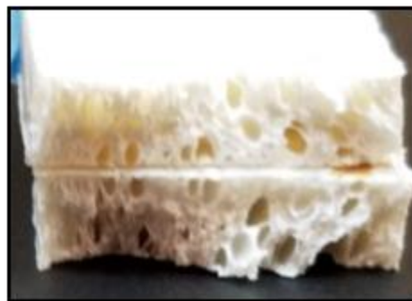
Figure 3.3: Cross-section of a macroporous CNF sample.
