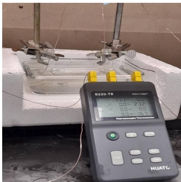
Figure 2. 2. Experimental setup for freezing point measurement.
