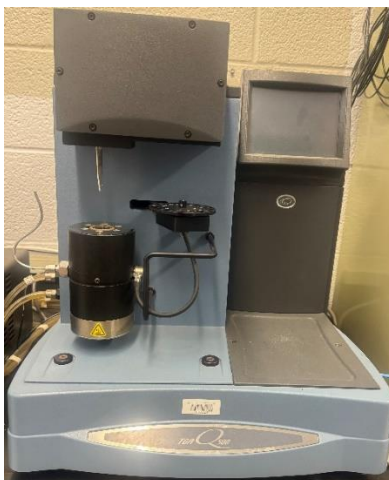
Figure 2. 5. The TGA Q500 used to study the mass loss of the parent kraft lignin and the obtained lignin fractions.
