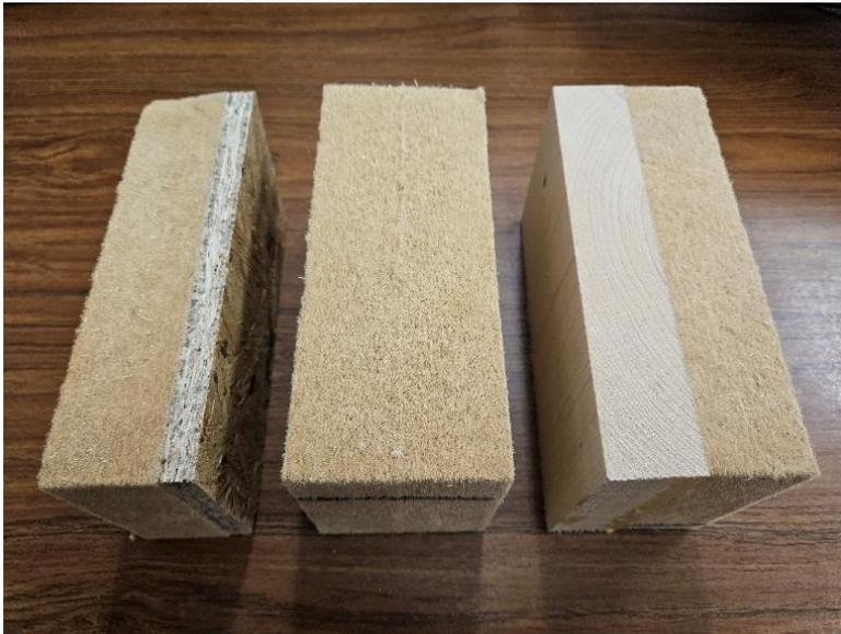
*Figure 1. 4: Test Panels Prior to Cutting (OSB, WFI, Lumber).*
