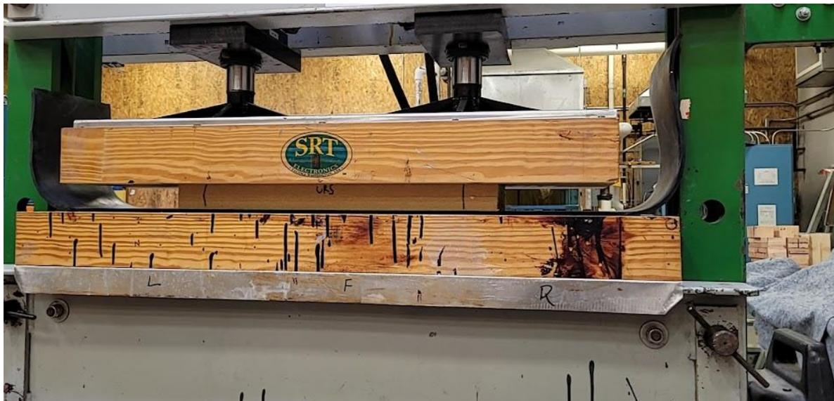
*Figure 1. 3: Hydraulic Press Being Used to Fabricate Test Samples.*
