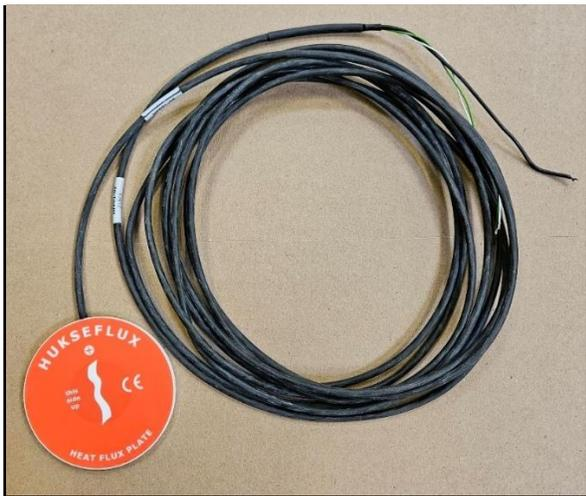
*Figure 2. 7: Hukseflux Heat Flux Sensor.*
