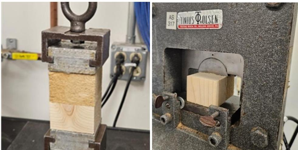
Figure 1. 5: Tensile (left) and Shear Testing (right) Fixture With a WFI:SPF Sample.
