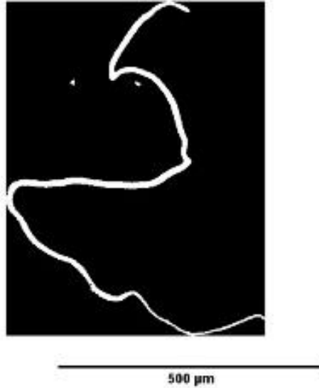
Figure 4: A sample image showing the thresholding program's output after background removal. The fiber is easily identifiable against the black background. The scale bar is 500 \mu\text{m} or 0.5 mm.
