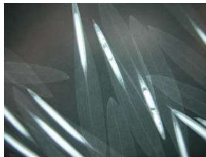
Close-up of X-ray of insect damaged ash seed.
