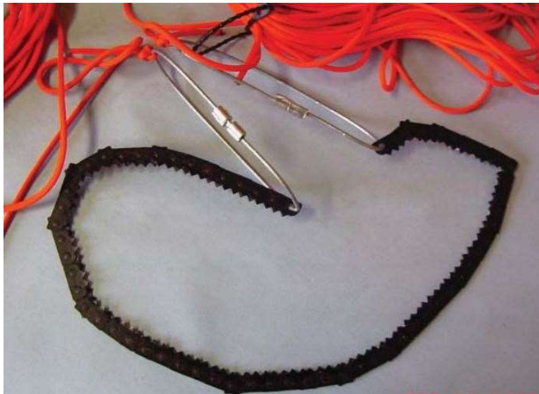
Figure 3.12. Example of a rope saw provided by US Forest Service (Mason, 2010).
