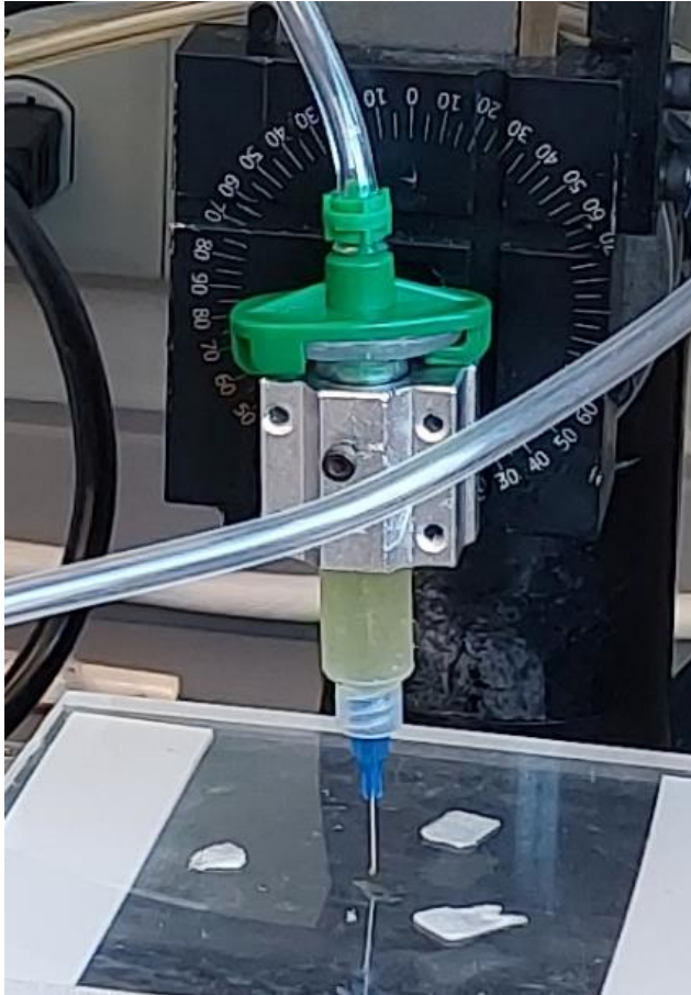
Figure 2.19. Dispense assembly of custom bioprinter at UMaine Digital and Additive Manufacturing Lab
