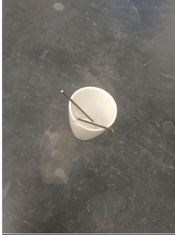
Figure 3-4: Anode Wires Inside a Crucible for Coating.
