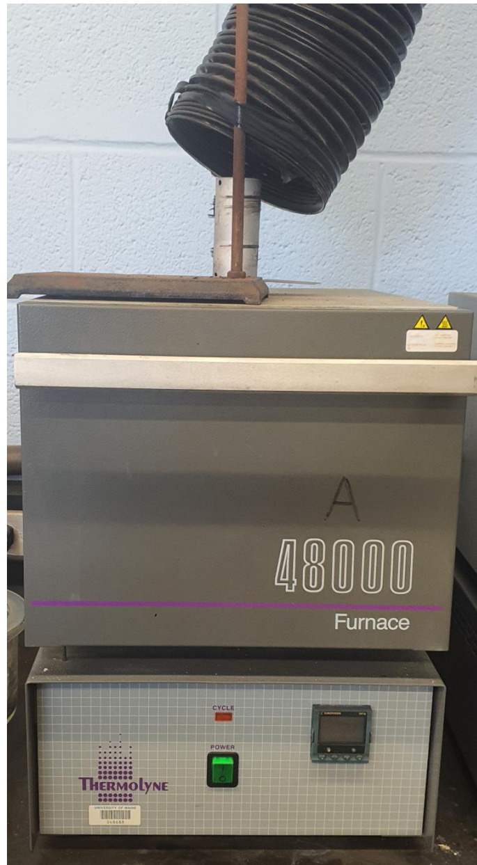
Figure 3-3: Furnace for annealing/coating processes.
