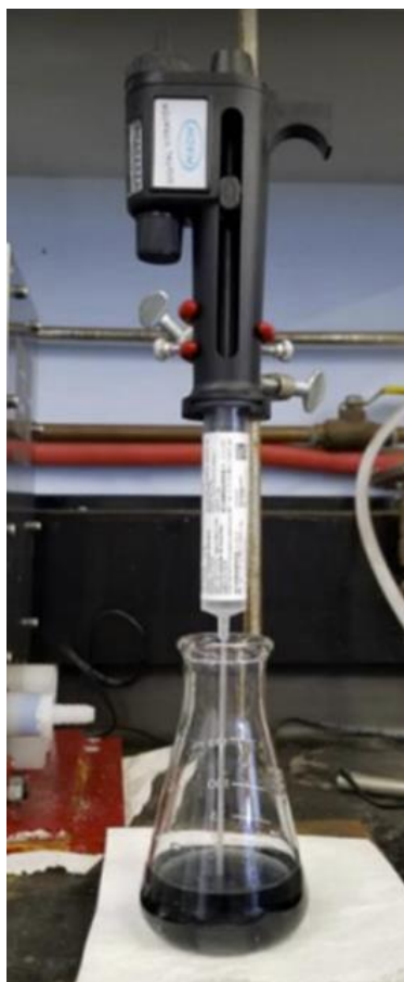
Figure 3-6: Hach Digital Titrator showing dark purple color before titration.
