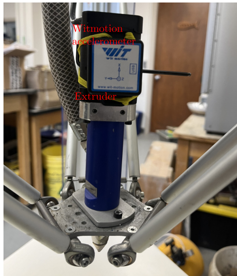
Figure A.1: Witmotion accelerometer attached to the extruder to measure printing time
