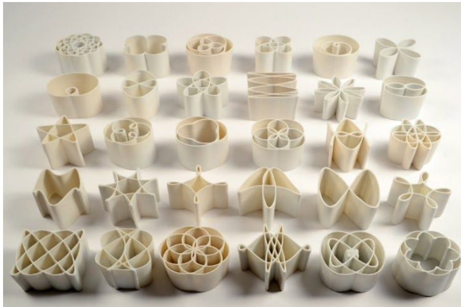
Figure 2.4: 3D printed objects from clay [3]
