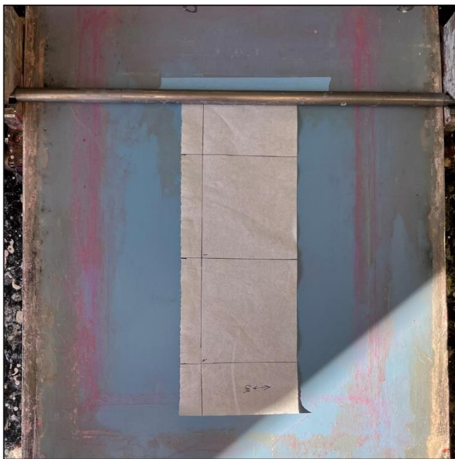
Figure 2.1. Uncoated substrate sample in the drawdown coating apparatus with the coating rod brought to the substrate/masking tape interface.
