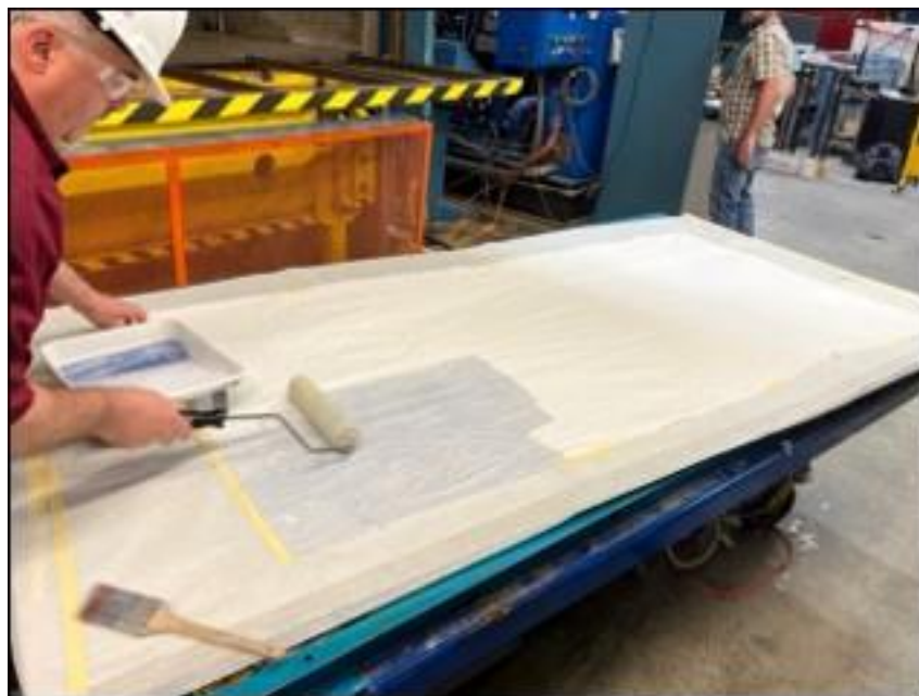
Figure 2.2. Hand roller coating of 3ft x 6ft paper substrate.
