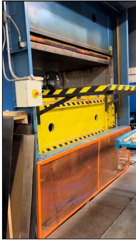
Figure 2.3. Image of Erie Mill & Press. The heated platen plate was actuated vertically according to instructions from a programmable logic controller.
