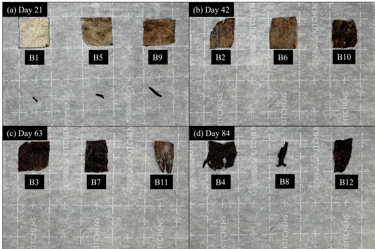
Figure 4.5. Appearances of composted UM39 (top row of each image) and paper substrate (bottom row of each image) samples removed from the windrow prior to drying. (a) 5cm x 5cm UM39 and paper substrate samples removed after 21 days in the windrow. (b) 5cm x 5cm samples removed after 42 days in the windrow. (c) 5cm x 5cm samples removed after 63 days in the windrow. (d) 5cm x 5cm samples removed after 84 days in the windrow.
