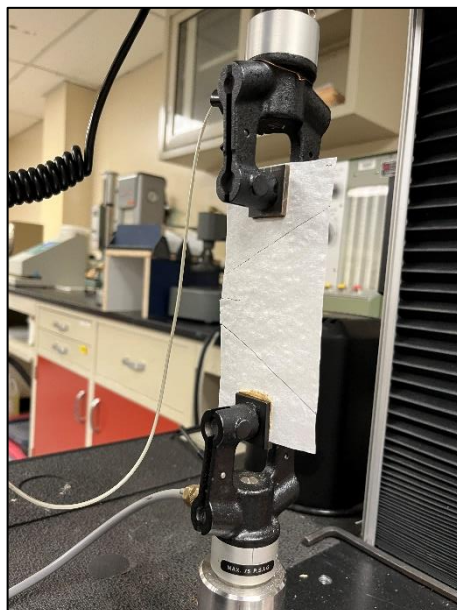
Figure 2.9. ASTM D5733 Test sample mounted in an Instron model 5564.
