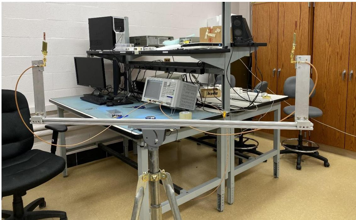
Figure 5.18: The NMHAS spaced 44 inches apart with the matching circuit connected.
