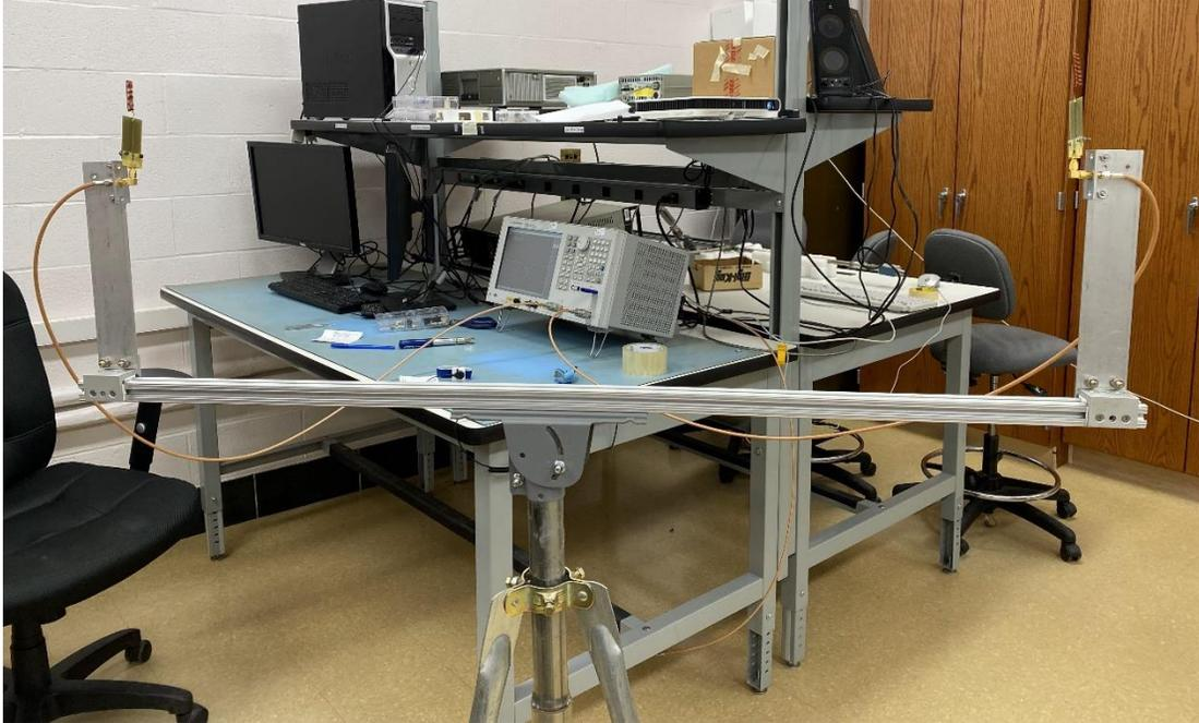
Figure 5.12: NMHAS mounted on antenna mounting structure and spaced 44 inches apart.
