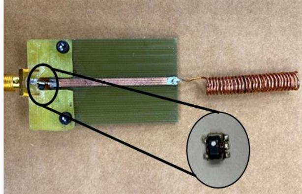
Figure 4.4: NMHAS balun connected at input.
