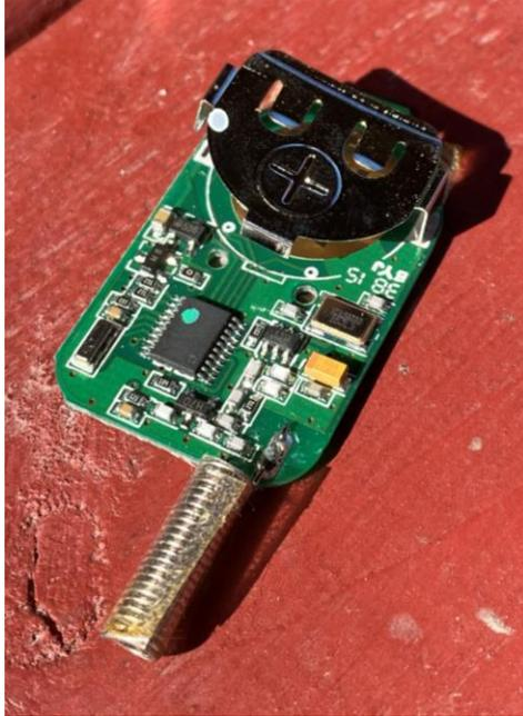
Figure 2.6: A car smart key with normal mode helical antenna connected to the circuit board.
