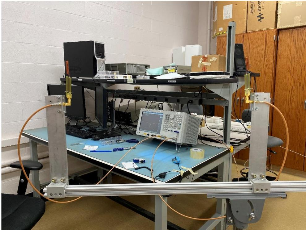
Figure 5.14: NMHAS mounted on antenna mounting structure and spaced 22 inches apart.
