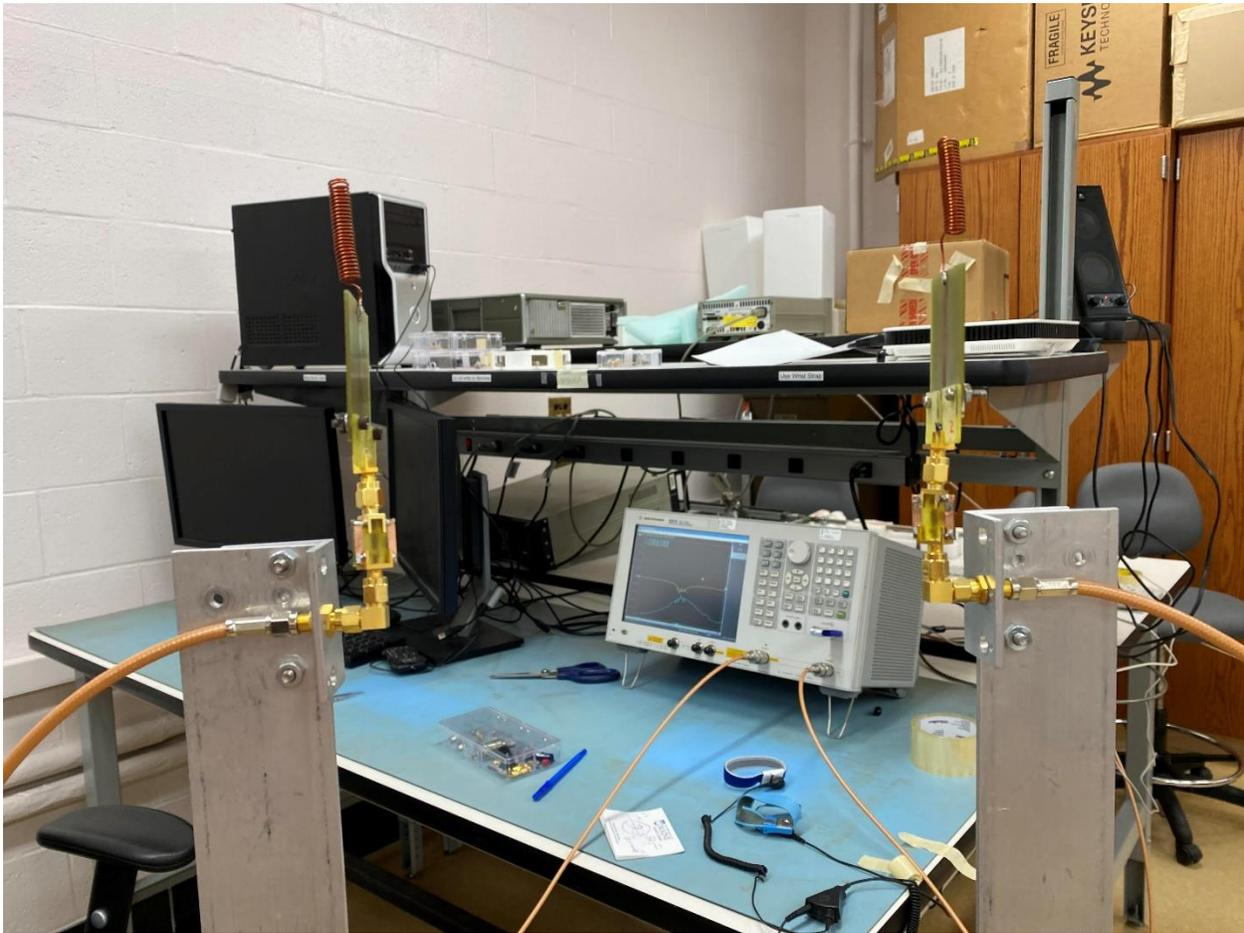
Figure 5.22: The NMHAS spaced 10 inches apart with the matching network connected.
