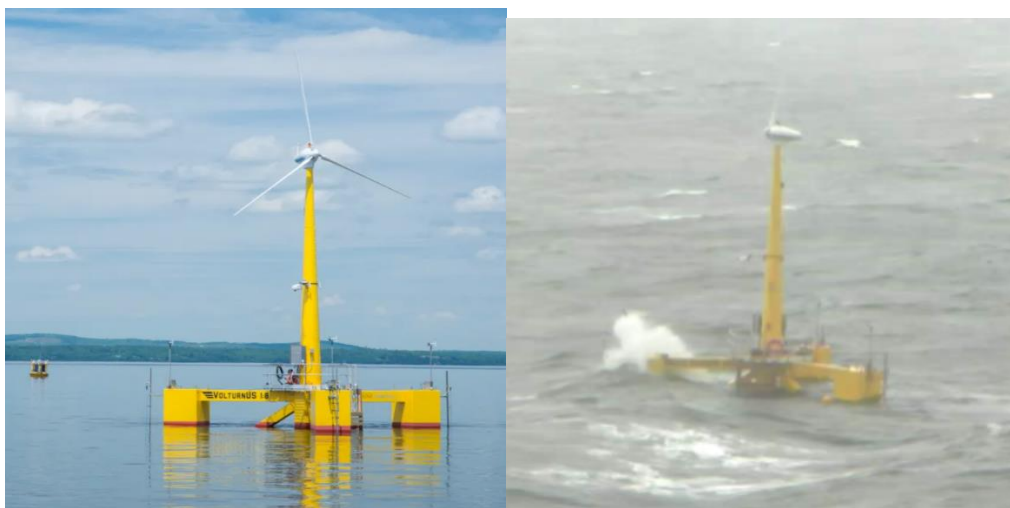
Figure 14: VoltturnUS 1:8 in Scaled Ocean Test Site in calm waters (left) and in an extreme environment (right). [23]
