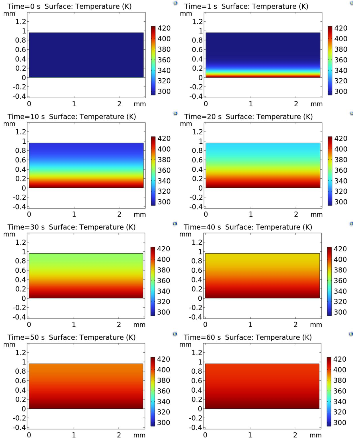
Figure 20. 2D images of temperature as a function of time for 240 μm paper. Red is high temperature and blue is low.
