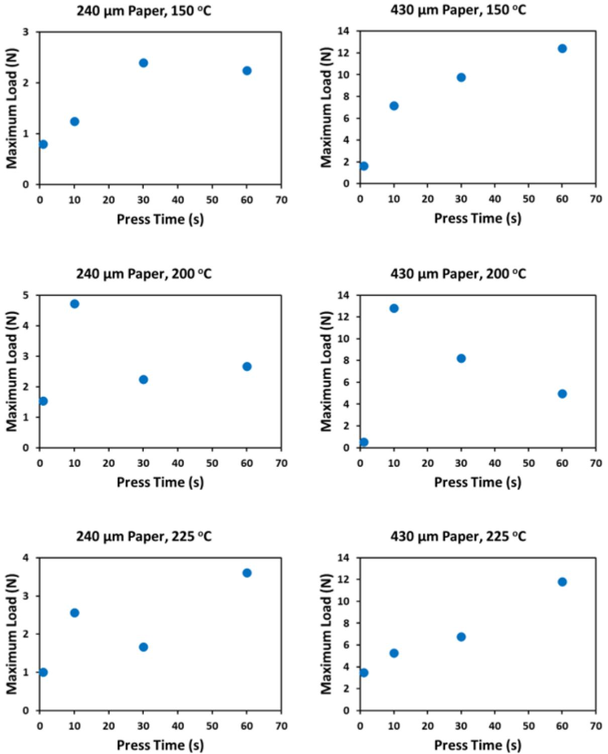
Figure 12. Tensile test results for 240 μm paper (left column) and 430 μm paper (right column) for 0.4 MPa press pressure.
