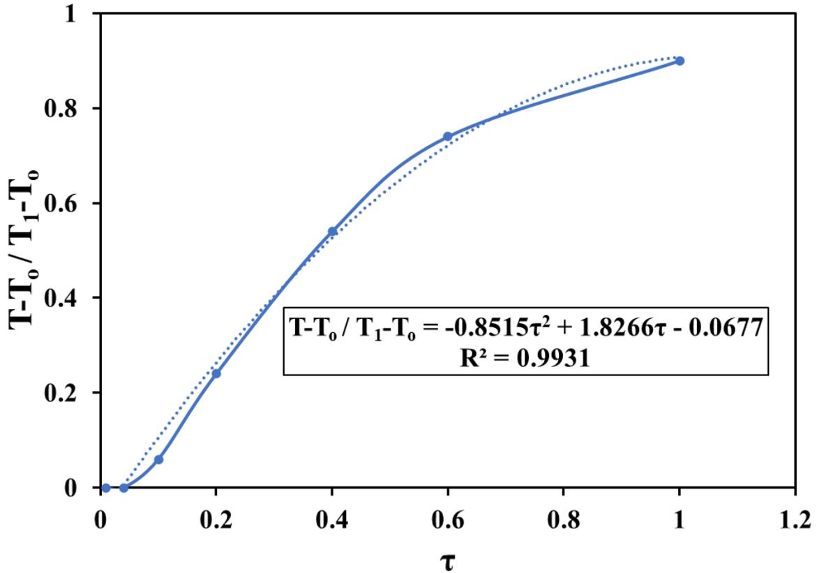
Figure 7. Temperature of the paper as a function of the press time.
