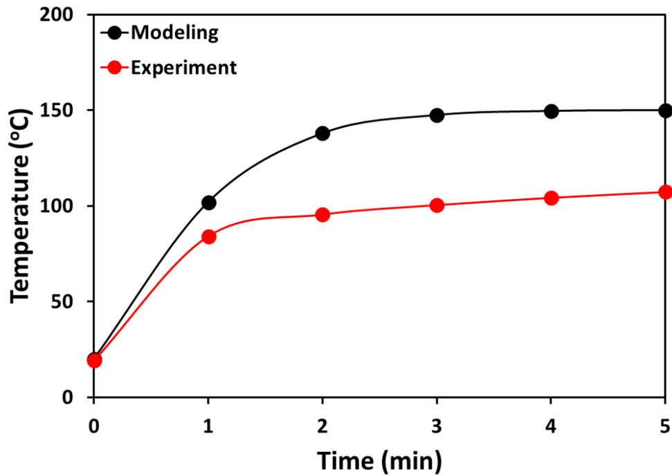
Figure 19. Comparing model predictions to the experiments for the 4-layers of 430  $\mu\text{m}$  paper.
