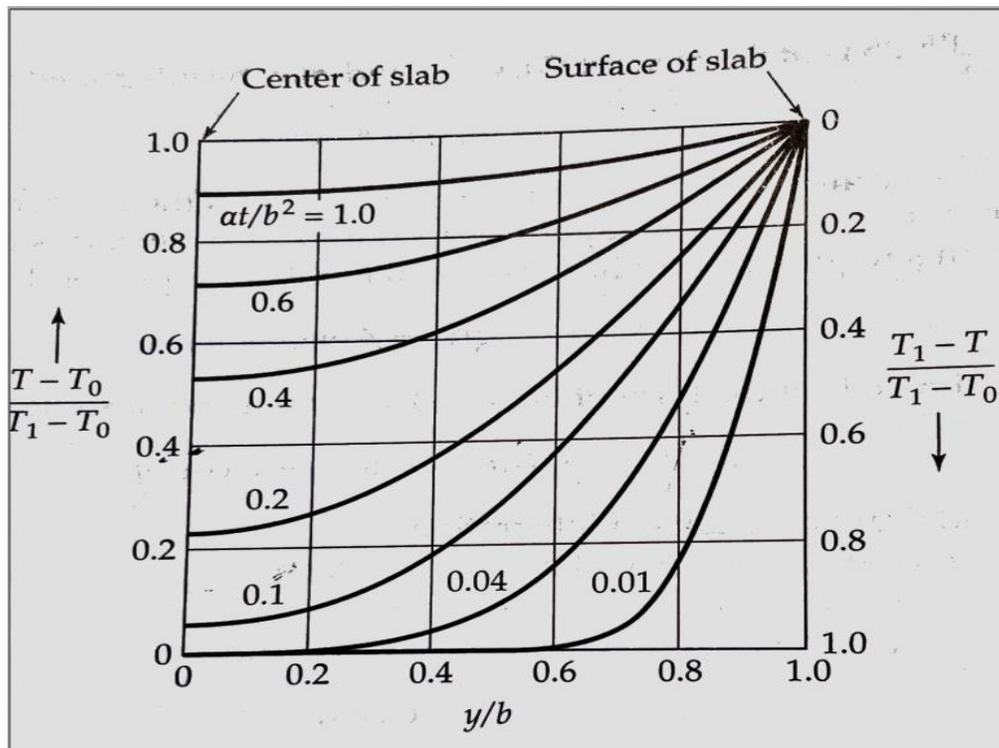
Figure 6. Temperature profiles for unsteady state heat conduction in a slab of finite thickness  $b$ . (H. S. Carslaw and J. C. Jaeger, conduction of heat in solids, 2<sup>nd</sup> edition, Oxford university press 1959, p. 101).
