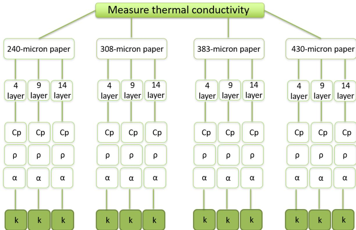
Figure 1. Scheme to measure the thermal properties of different papers.
