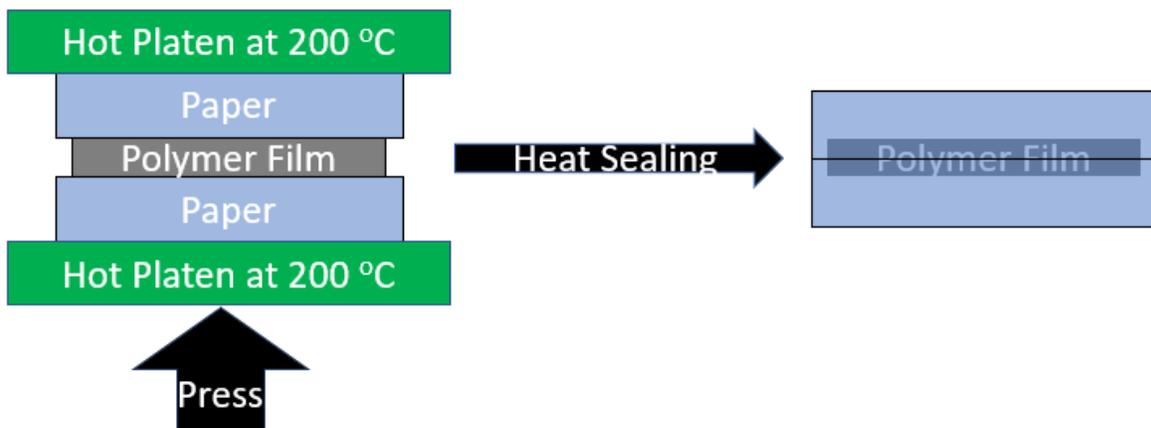
Figure 10. Heat sealing process using carver press method.
