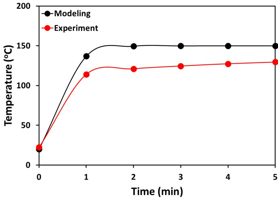
Figure 17. Comparing model predictions to the experiments for the 4-layers of 308  $\mu\text{m}$  paper.
