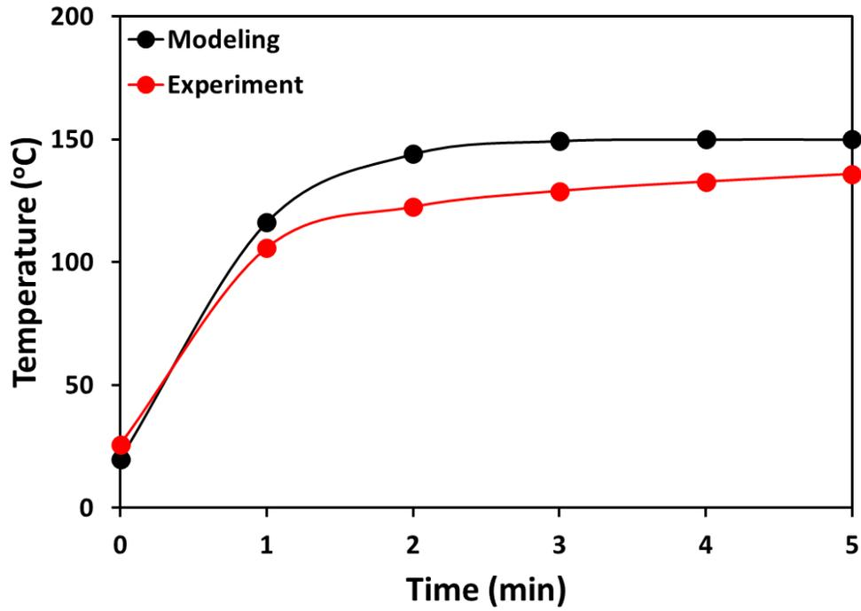
Figure 18. Comparing model predictions to the experiments for the 4-layers of 383  $\mu\text{m}$  paper.
