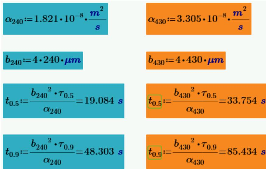
Figure 9. Time required for two different papers of four layers each to reach half of the platen temperature or the platen temperature itself using 0.4 MPa press pressure in carver press method.
