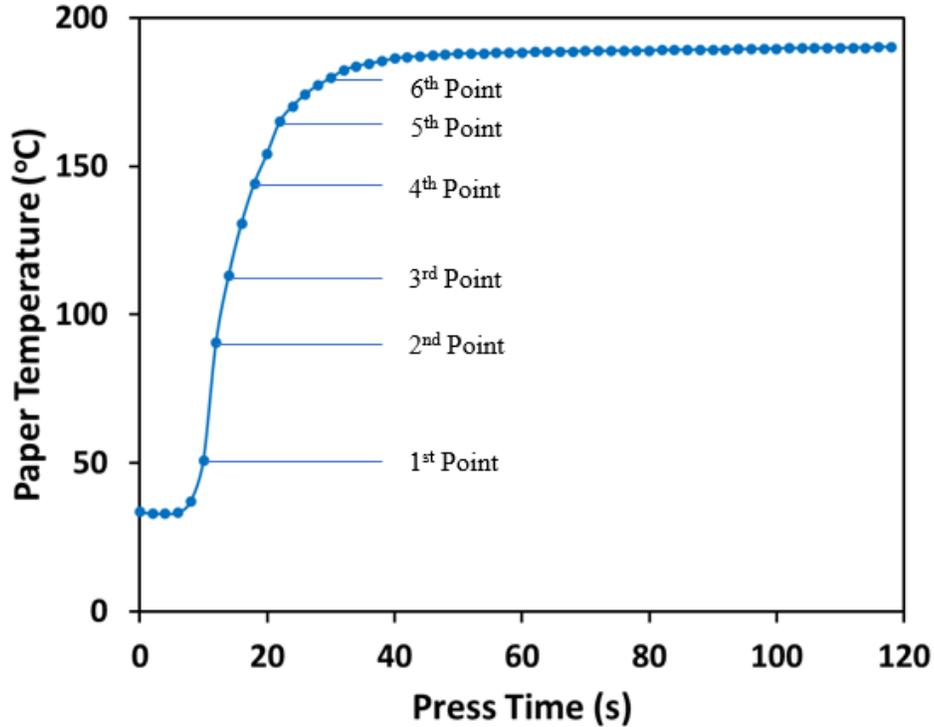
Figure 5. Paper temperature as a function of press time for the four-layers 240  $\mu\text{m}$  paper type pressed at 0.4 MPa in the carver press method.
