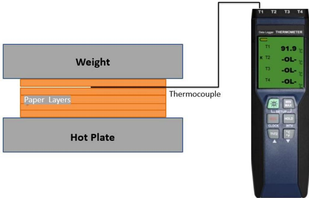
Figure 4. Measuring temperature increase as a function of time in four layers of a paper using the hot plate method.
