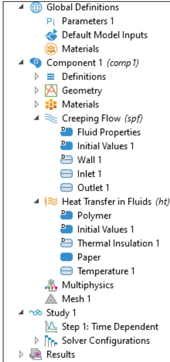
Figure 23. Tree properties for the polymer flow into the paper as well as heat transfer.
