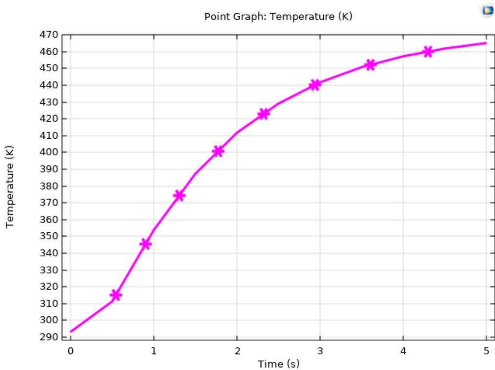
Figure 27. Surface temperature of polymer as a function of time for the 430  $\mu\text{m}$  paper.
