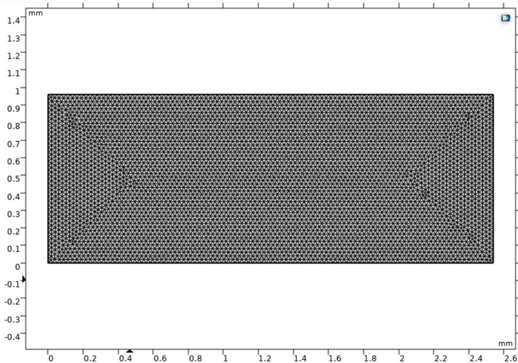
Figure 13. Paper geometry in 2D coordinate meshed system.
