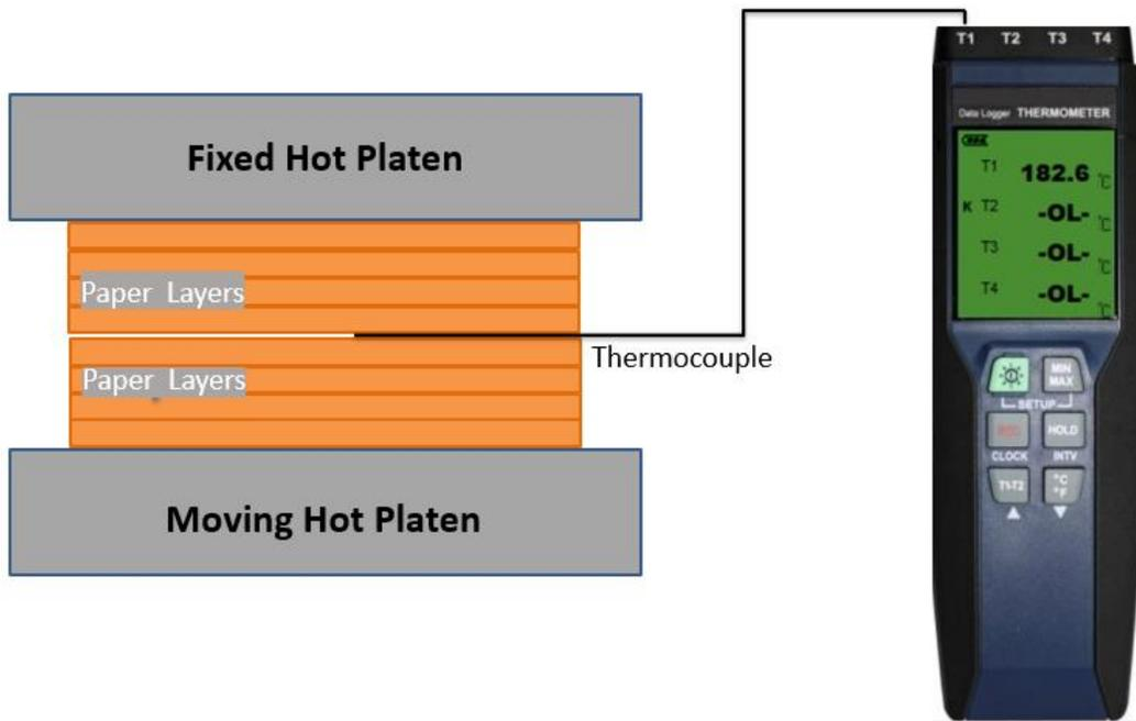
Figure 3. Measuring temperature increase as a function of time in four layers of a paper using the carver press method.
