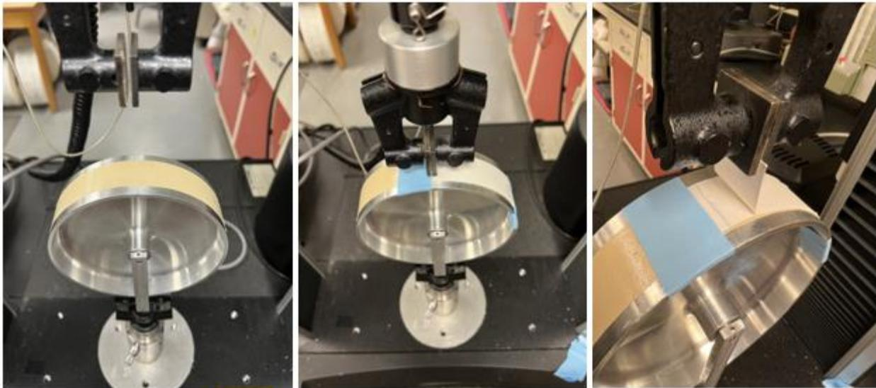
Figure 11. Peeling test to separate two glued samples.
