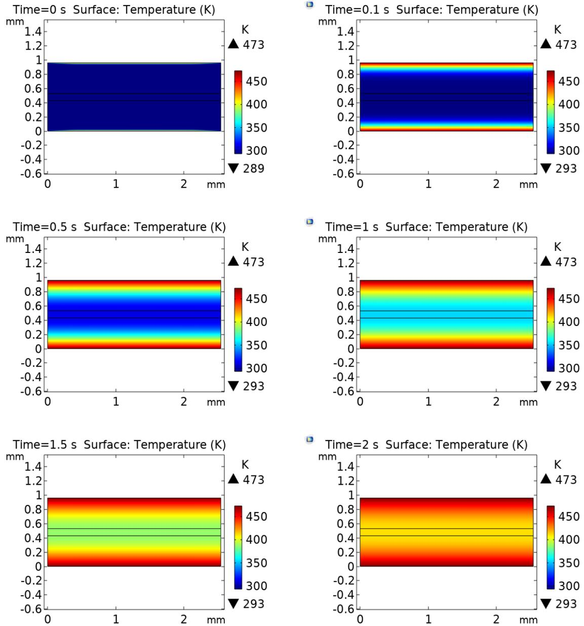
Figure 25. 2D images show how the temperature transferred through 430  $\mu\text{m}$  papers into the polymer layer as a function of time. Red is high temperature and blue is low..
