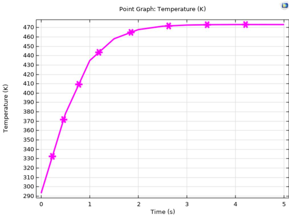
Figure 26. Surface temperature of polymer as a function of time for the 240  $\mu\text{m}$  paper.
