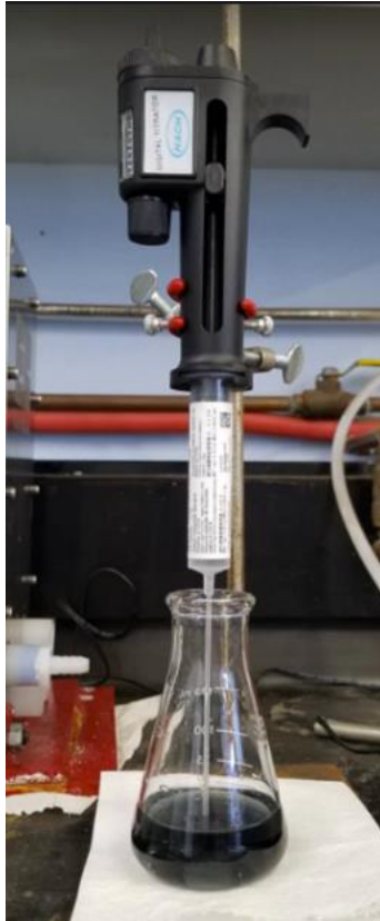
Figure 6. Hach Digital Titrator showing color before titration.
