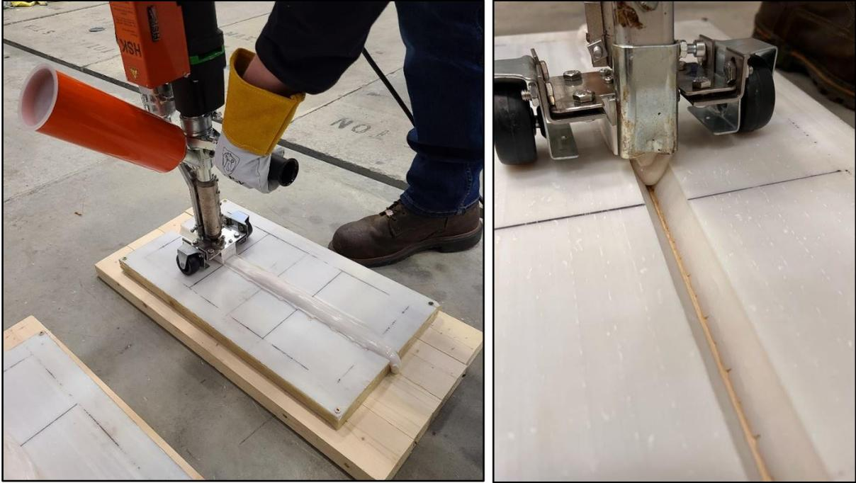
*Figure 22: Extrusion Welding AM Plate*
