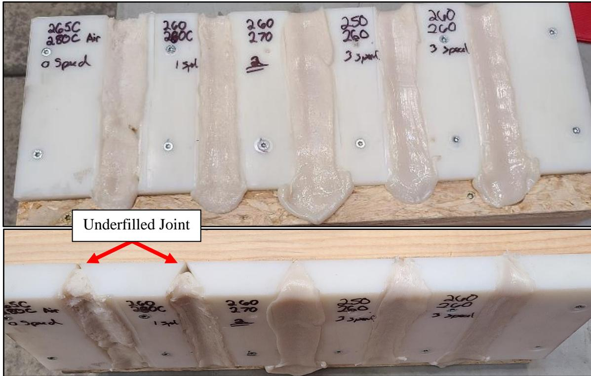
Figure 15: Extrusion Welds conducted for Welder Calibration.
