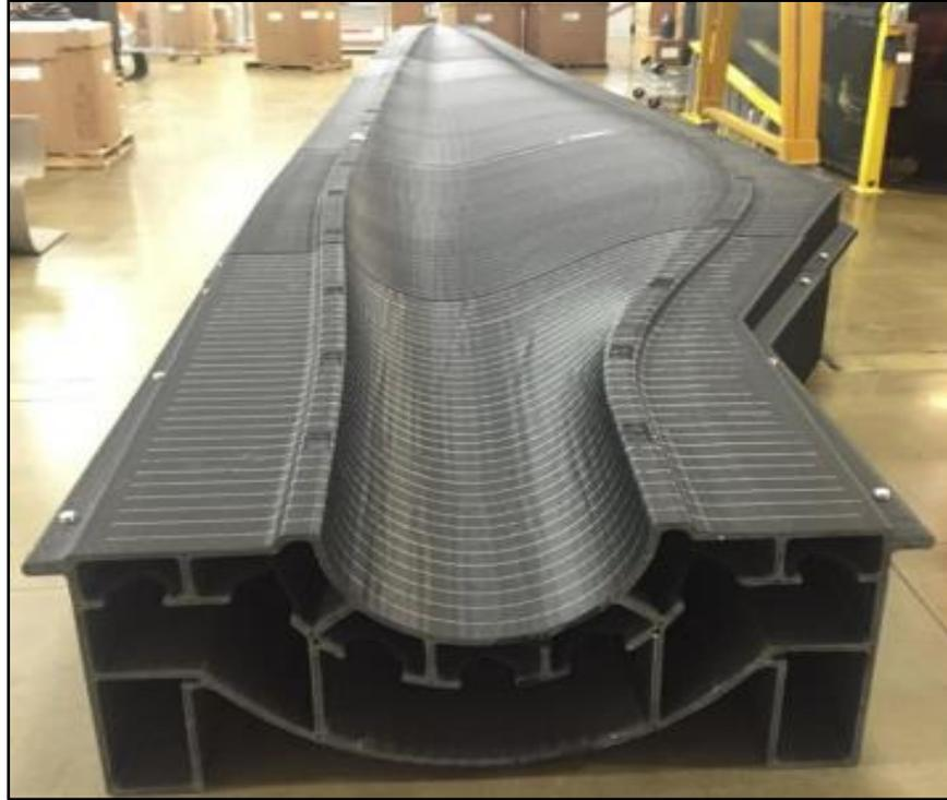
*Figure 4: ORNL & TPI Inc. 2017 - AM of Wind Turbine Molds [2]*
