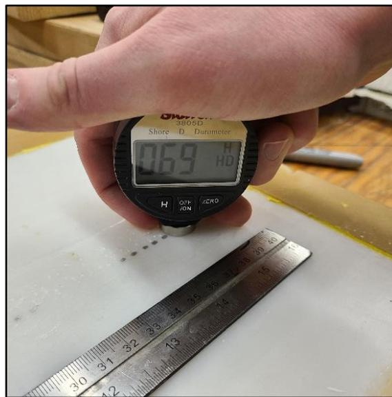
*Figure 36: Starrett 3805D Shore D Durometer in use on weld*
