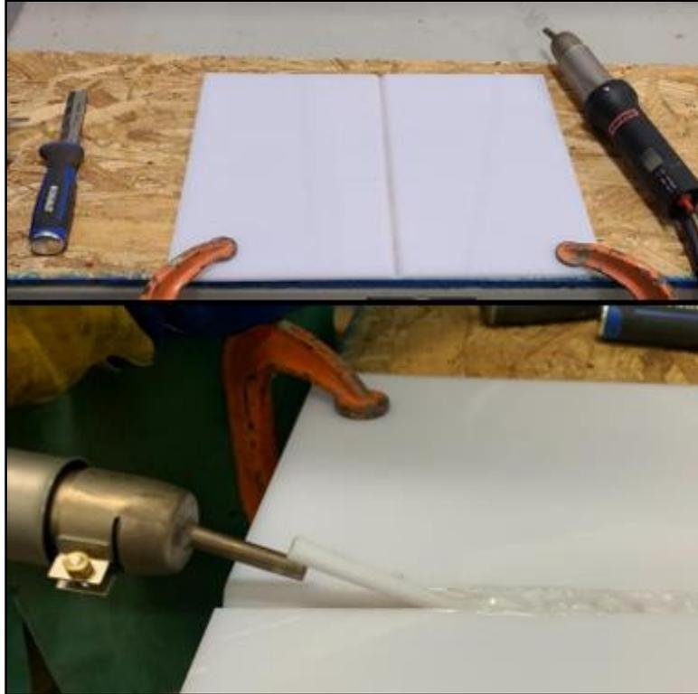
*Figure 8: Set-up and Initial Hot Gas Pendulum Weld*
