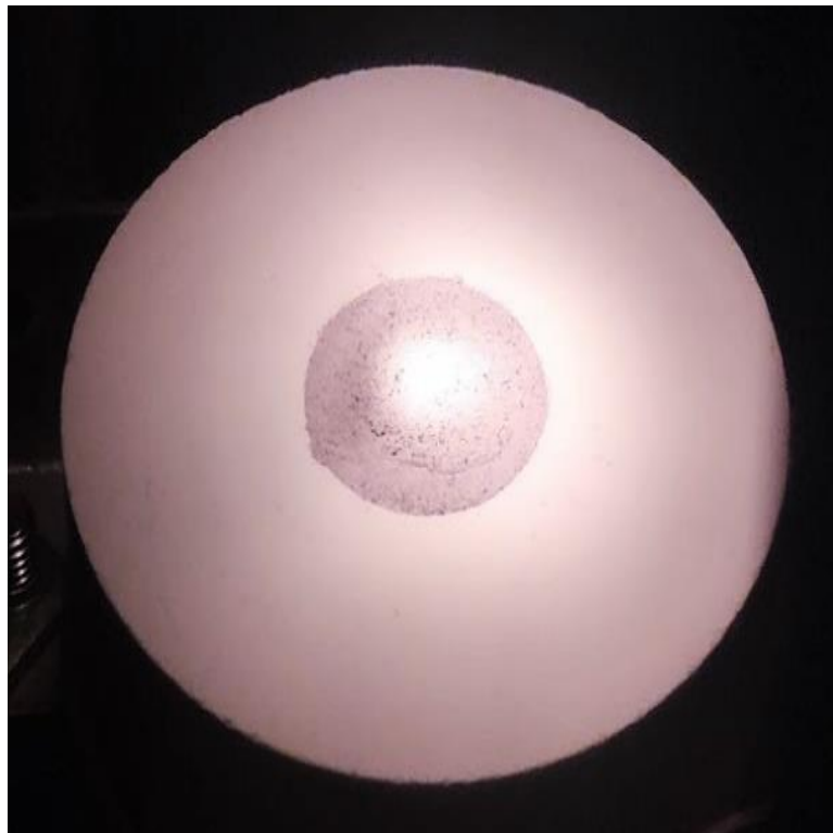
Figure 2.3. LHS-1 bed of 30 mm radius under direct concentrated irradiation
