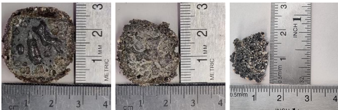
Figure 4.10. Sintered pieces at 0 mm distance for 80 A, 70 A, and 60 A input currents
