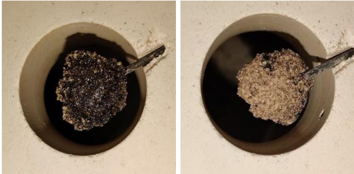
Figure 3.10. Attached sintered material with top thermocouple at 70 mm distance and 60 A input current
