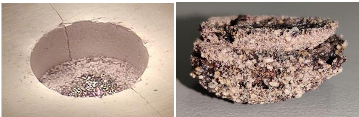
Figure 3.29. Layer by layer sintering with sintered pieces of three 3 mm layers
