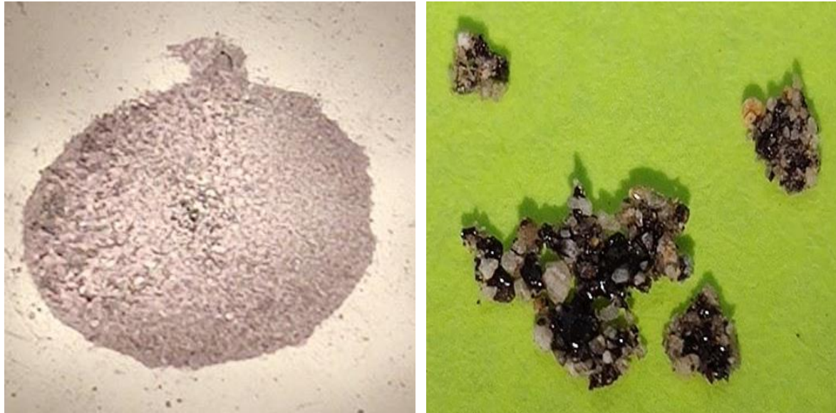
Figure 3.8. Sintering started at 135 mm distance for 60 A current
