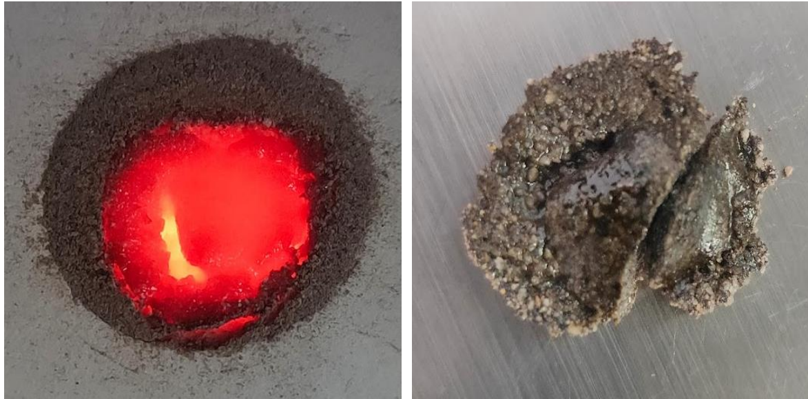
Figure 3.5. Melted lunar soil simulant and broken sintered part at 60 mm distance
