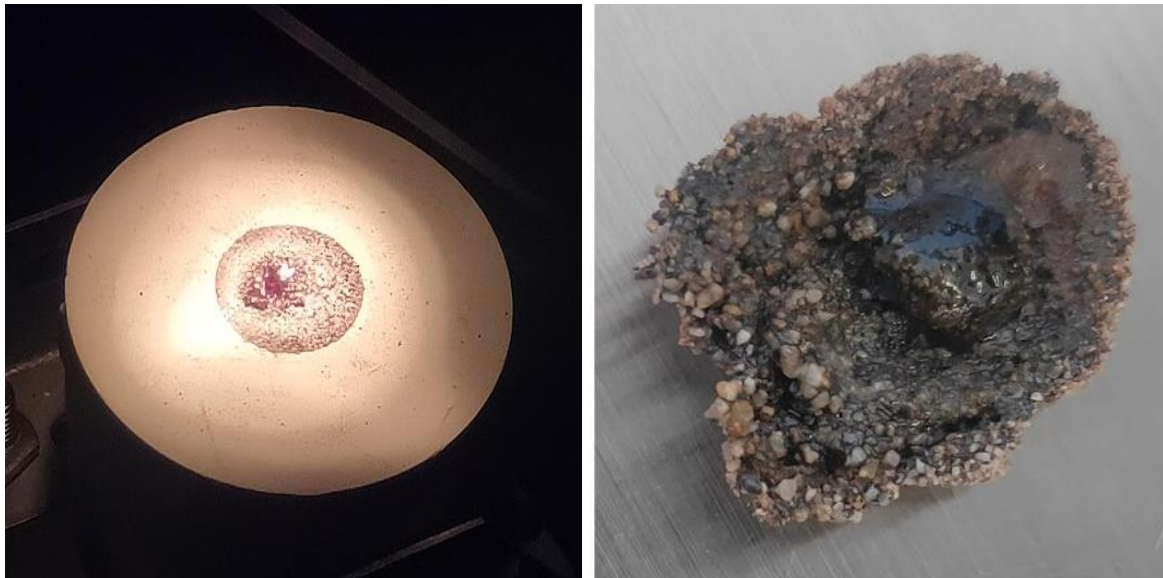
Figure 3.4. Melted simulant at 80 mm distance and 60 A current
