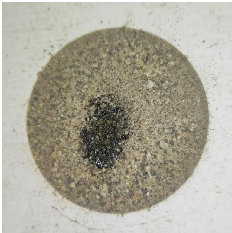
Figure 3.3. Sintered LHS-1 on the simulant bed at 130 mm distance and 60 A current
