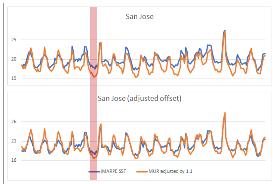
Figure 2.10: San Jose in-situ and MUR records (top) and in-situ and MUR records after MUR data was adjusted by 1.1°C (bottom). Vertical line indicates the 2007-2008 La Niña event.
