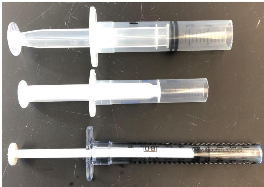
Figure 3.1: Size comparison of 5 mL, 3 mL, and 1 mL cut-off syringes used as molds for forming hydrogels. The syringe sizes from top to bottom are: 5 mL, 3 mL, and 1 mL.
