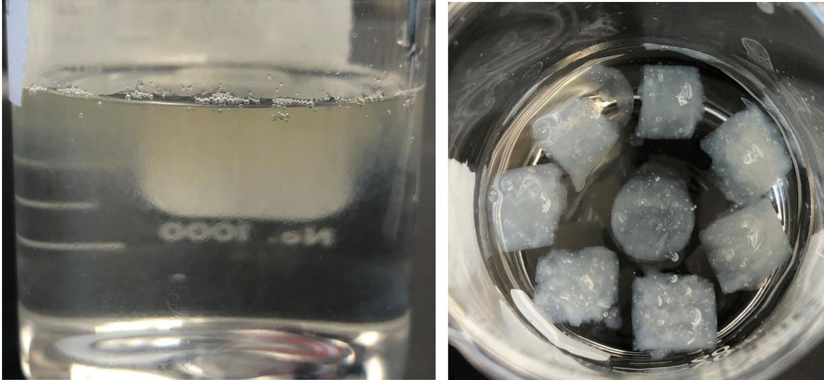
Figure 3.2: Failed attempt at mixing TEMPO CNF and bacterin where it dispersed in citric acid solution (left). Successful attempt at forming hydrogels from TEMPO CNF and bacterin mixture using a 3 mL cutoff syringe (right).
