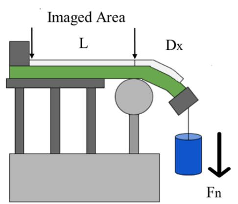
Figure 3. 1. Schematic of the unilateral stretching force apparatus for aligning CNF samples using constant uniaxial force
