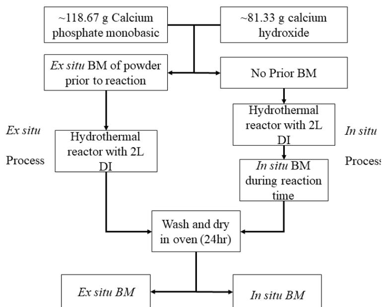
Figure2. 1Process flow diagram for hydrothermal synthesis of
