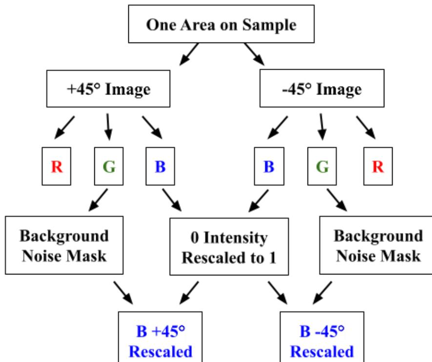
Figure 3. 1. BOI calculation process flow chart.
