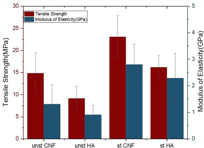
Figure 3. 8. Tensile strength and modulus of elasticity of films
