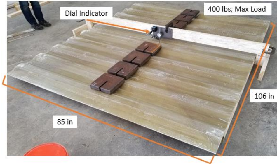
Figure 9: Sidewall Panel Three-Point Bending Test Loaded
