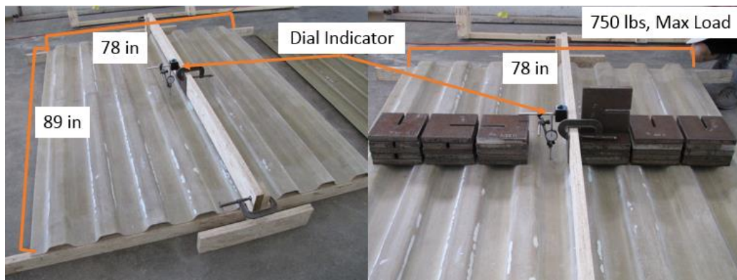
Figure 10: Frontwall Panel Three-Point Bending Test, Unloaded (Left), Loaded (Right)
