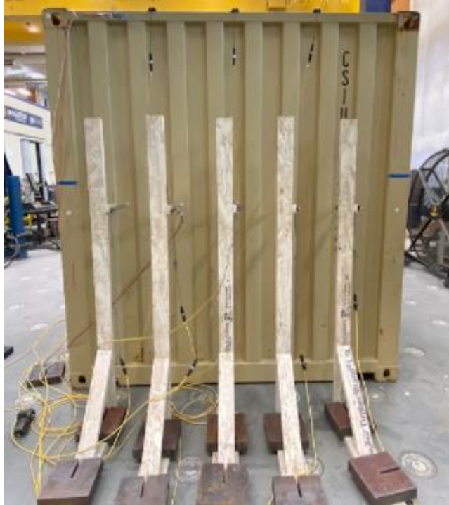
Figure 36: Frontwall Strength Test Setup
