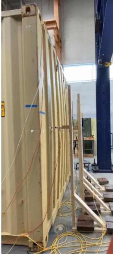
Figure 37: Frontwall Strength Test Loaded
