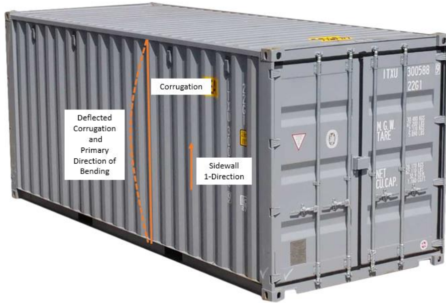
Figure 5: Primary Direction of Bending of Panels
