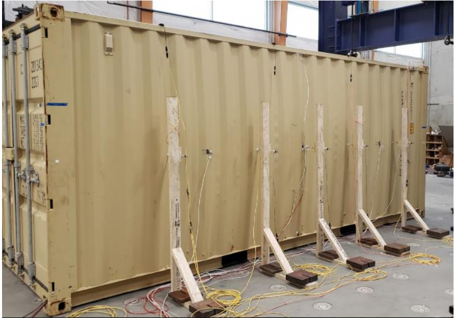
Figure 20: Sidewall Strength Test Loaded
