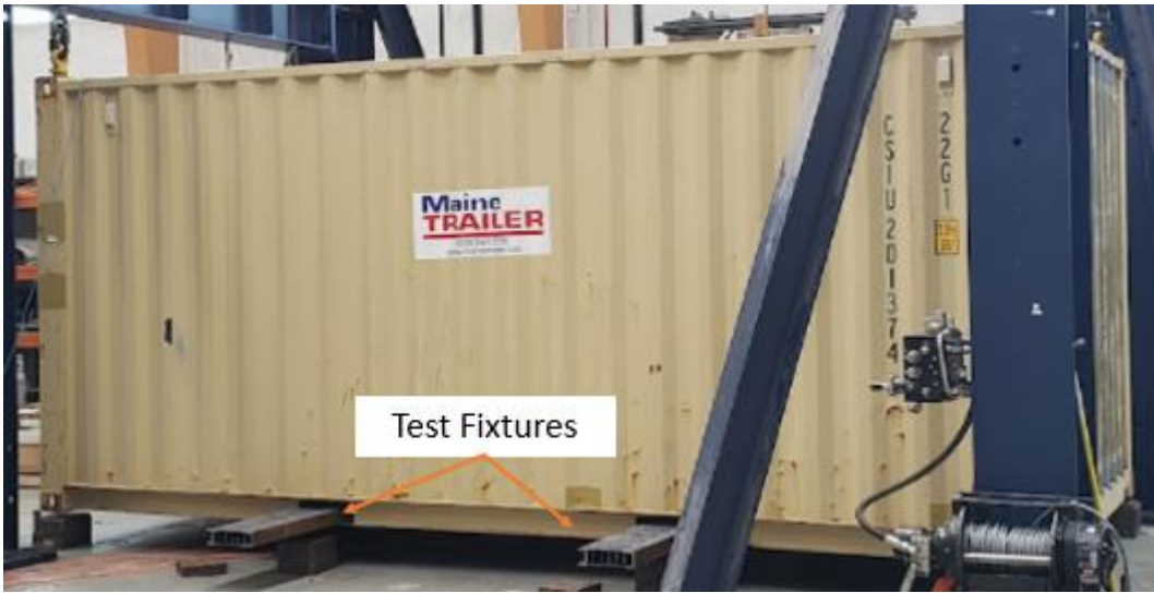
Figure 42: Fork Pocket Test Setup
