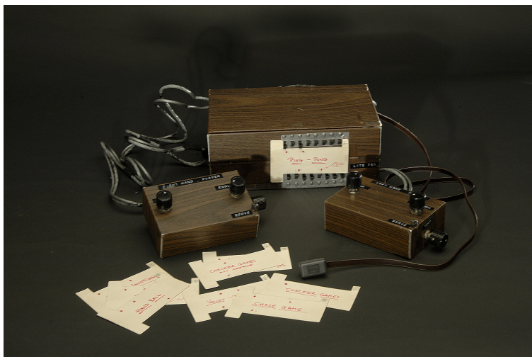
Figure 2.4: Photo of the Brown Box with program cards.
