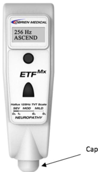
*Figure 5.1: Electronic Tuning Fork utilized in this thesis, the device is 12 inches long and fits in your hand. The device is used for measuring diabetic foot neuropathy and the cap (indicated in figure) is placed on the bottom of your foot.*
