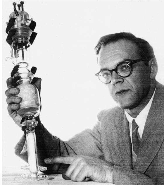
*Figure 2.9: Lenard Clark with his invention of defoaming in an oxygen bubbler that helped construct the Clark electrode. Image replicated from [30]*
