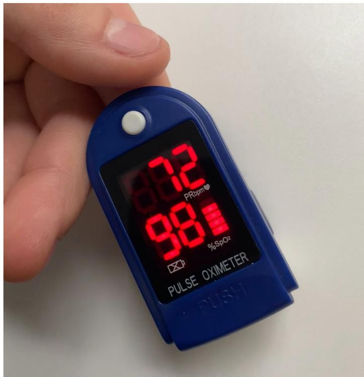
*Figure 2.10: Finger pulse oximeter, most commonly used in hospitals, the device is placed over the finger to read heart rate and blood oxygen saturation.*
