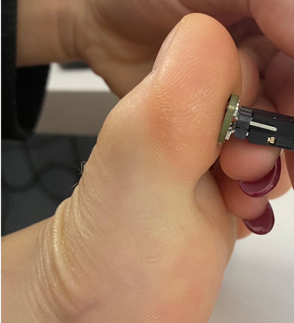
*Figure 6.1: Designed PPG sensor placed on the bottom of the big toe in the study for testing.*
