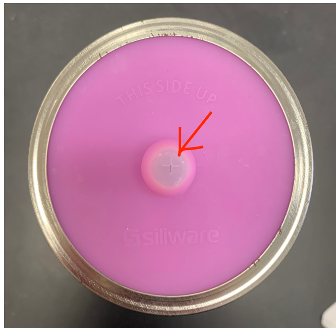
Figure 2.3. The opening on the silicon fermentation lid used for sample extraction to reduce the introduction of oxygen and contamination
