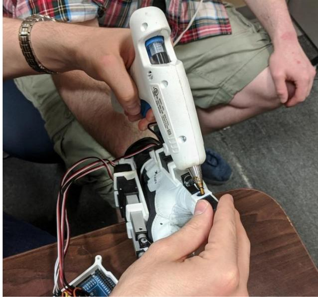
Figure 4.12 The steel strip for the thumb being fixed to the thimble.
