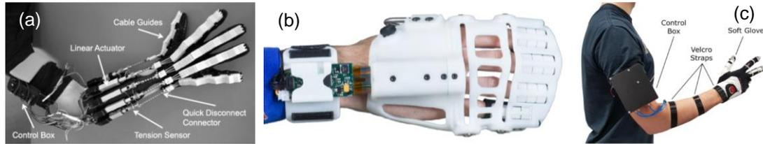
Figure 1.5 Examples of wearable control systems mounted on the (a) upper arm [3], (b) wrist [8], and (c) again on the upper arm [25].
