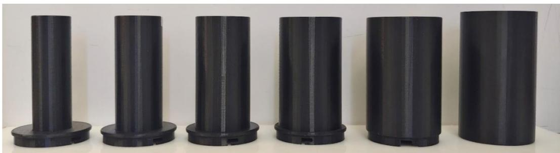
Figure 3.5 The container used for testing (far right) and the different caps. From left to right, the cap diameters are 40mm, 50mm, 60mm, 70mm, and 80mm. The container is also 80mm in diameter.
