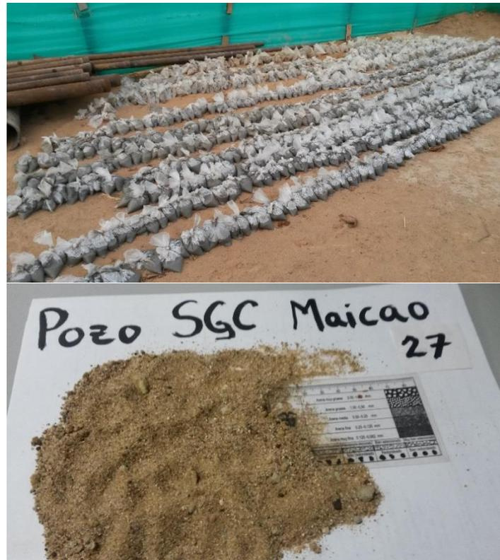
Figure 11. Elements for generating the sedimentary columns. **Left:** Schematic diagram of Gamma ray (GR), Spontaneous potential (SP), and Resistivity logging (RES) relative responses in consolidated rocks (modified from Todd, 1959). **Right Top:** well cuttings taken at 1 m intervals from a rotary-drilled well in Maicao collected in 2013. **Right Bottom:** 27 m deep well cutting sample after being washed and dried.
