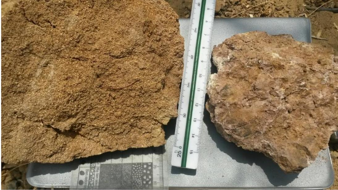
Figure 7. Hand samples of the predominant lithologies in the Monguí Formation. Samples collected 3 km away from Maicao. Lithic sandstone (**right**) and calcareous claystone (**left**).
