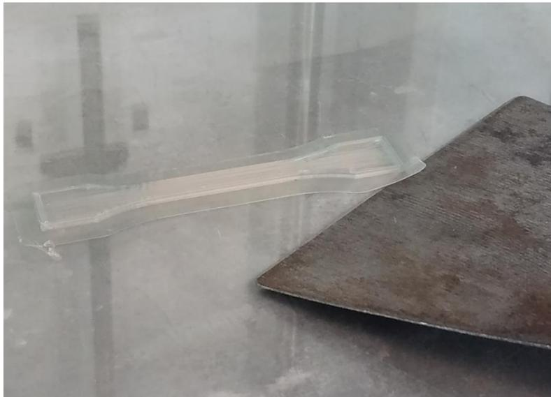
Figure 21: Removal of a clear PLA ½-scale D638 tensile dog bone specimen with putty knife
