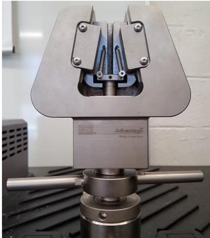
Figure 25: MTS Advantage wedge-action grips
