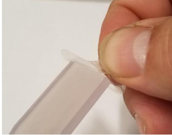
Figure 22: The folding-and-peeling process, removing brim rasters from a tensile specimen
