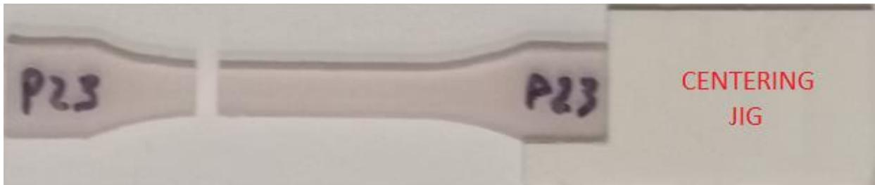
Figure 24: The fitment of a tensile specimen to the centering jig
