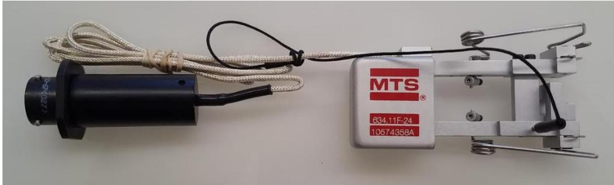
Figure 26: The 25-mm extensometer used for testing
