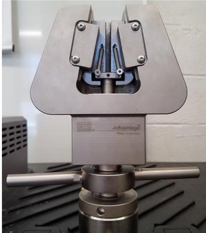
Figure 25: MTS Advantage wedge-action grips
