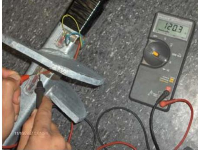
Figure 2.24. Strain gages installed on square shaft helical anchors (Abdelghany and El Naggar 2010)
