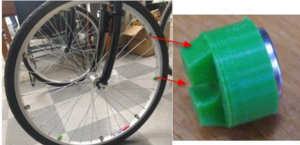
Figure 2.20: Placement of magnets on wheel on the left and close-up of magnet in 3D printed holder on the right.
