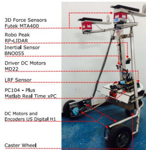
Figure 1.9: Smart walker fitted with multiple sensors and CPU (Jiménez et al, 2018)
