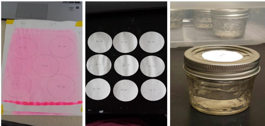
Figure 2.1.2 Procedure for sample forming and WVTR measurement apparatus.
