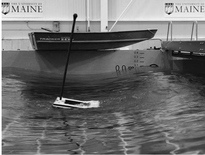
Figure 2.7. Overtopping during regular wave 4
