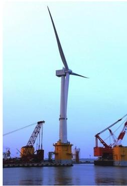
Figure 1.7. Fukushima Shimpuu, fabrication complete (Mitsubishi Corporation, 2015)
