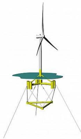
Figure 1.10. Deployed Tetraspar (Lauridsen, 2017)
