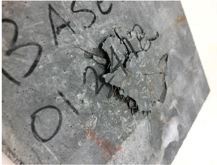
Figure 5.10. Damage to an Elium-reinforced panel from quasi-static loading
