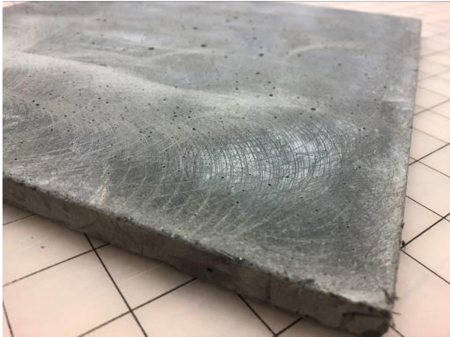
Figure 3.9. Roughened UHPC surface
