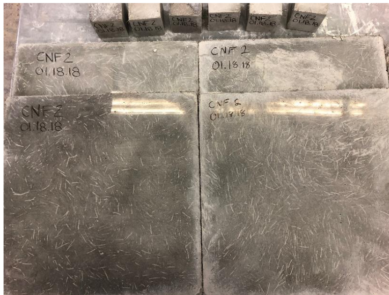
Figure 3.3. Panels and cubes after demolding
