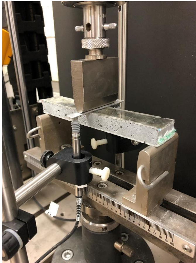
Figure 4.4. Beam test setup on a 5kN Instron machine
