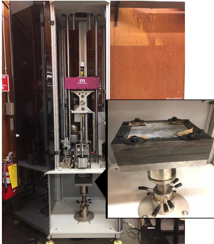
Figure 5.4. Instron 9350 CEAST Drop Tower test setup
