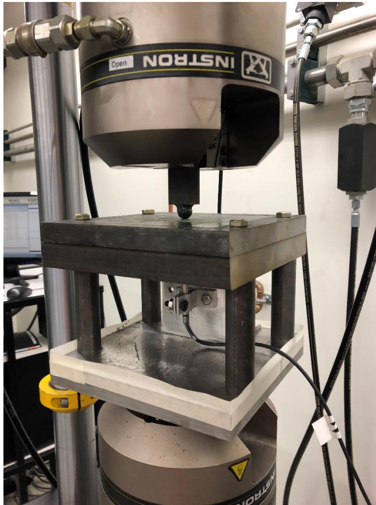
Figure 5.3. Quasi-Static test setup on a 100kN Instron machine
