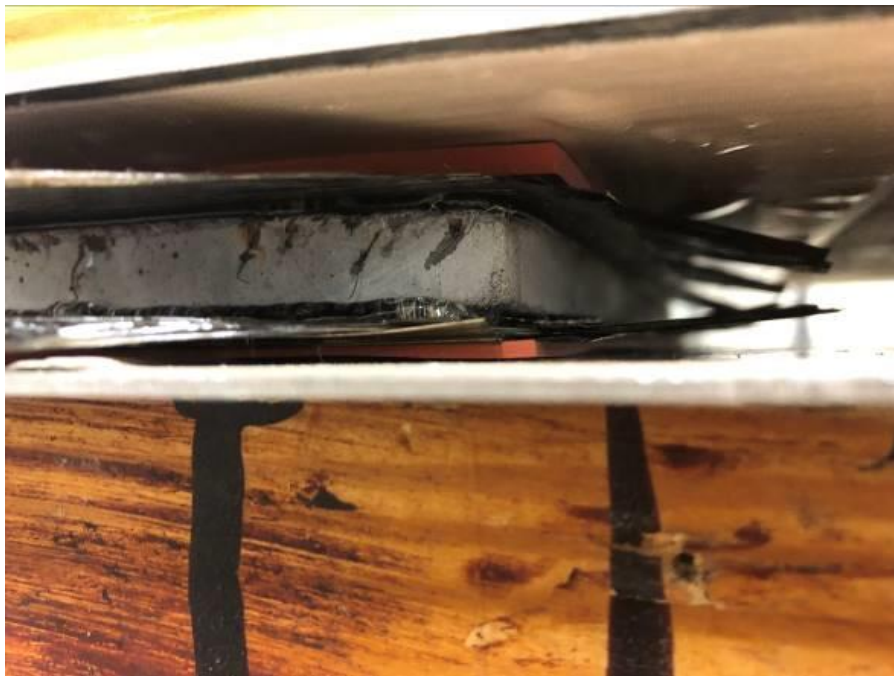
Figure 3.11. Double-sided PETg panel during fabrication
