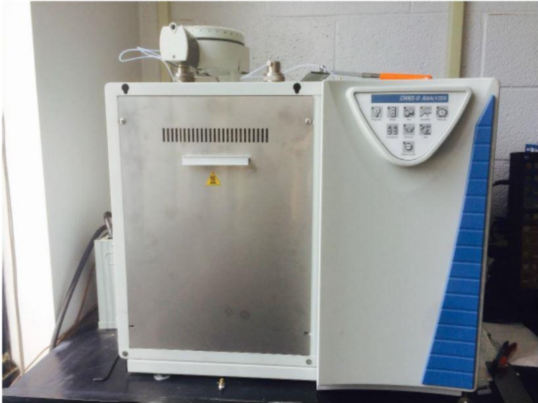
Figure A.1 Elemental analyzer for CHNO
