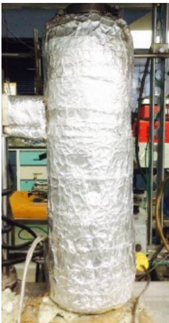
Figure 4.4 Hot gas filter unit
