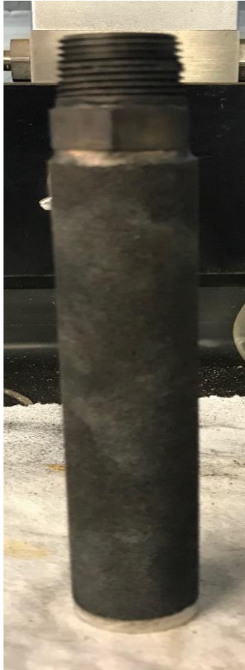
Figure 4.3 Hot gas filter
