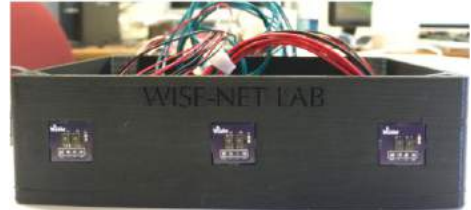
(b) UMaine's WLD System, Dimensions 18cm by 13cm by 7cm.
