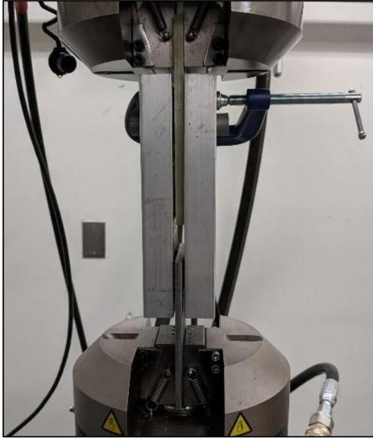
Figure 84: TP Stud Shear Testing Custom Fixture
