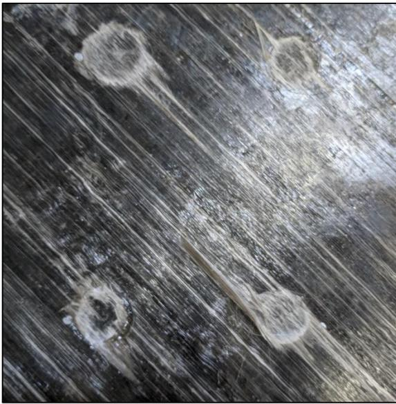
Figure 102: Failed PETg Concrete-TP Stud
