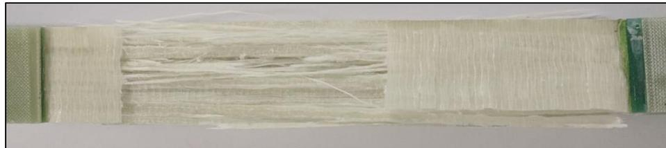
Figure 21: Feasibility E-glass/Elium XGM Failure Long. Tension Sample
