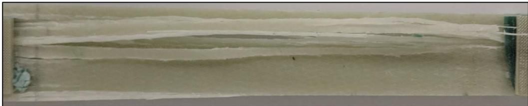
Figure 46: E-glass/Elium UD DGM Failure Long. Tension Sample
