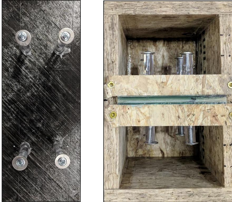
Figure 96: Concrete-TP Specimen Plate & Formwork
