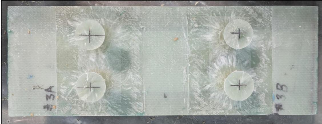
Figure 82: E-glass/Elium Shear Stud Infusion Result
