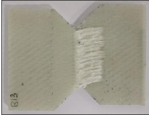
Figure 23: Feasibility E-glass/Elium HGN Failure In-Plane Shear Sample
