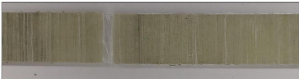
Figure 32: E-glass/PETg UD Failed Trans. Tension Sample
