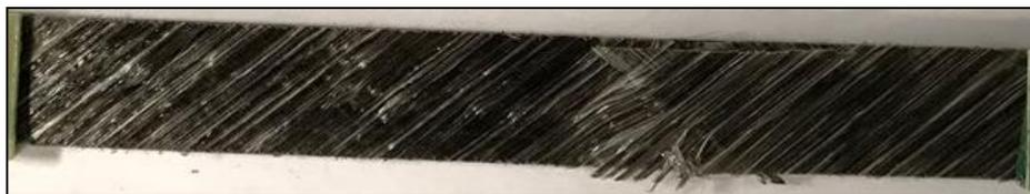
Figure 64: E-glass/PETg [+/- 45 90 0]s Failed Tension Sample
