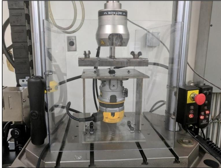
Figure 73: Instron Welding Setup
