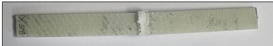
Figure 22: Feasibility E-glass/Elium BGM Failure Long. Compression Sample
