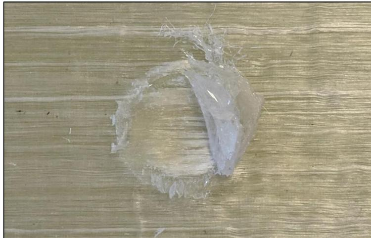
Figure 90: Failed Instron Welded Single TP Stud Shear Specimen
