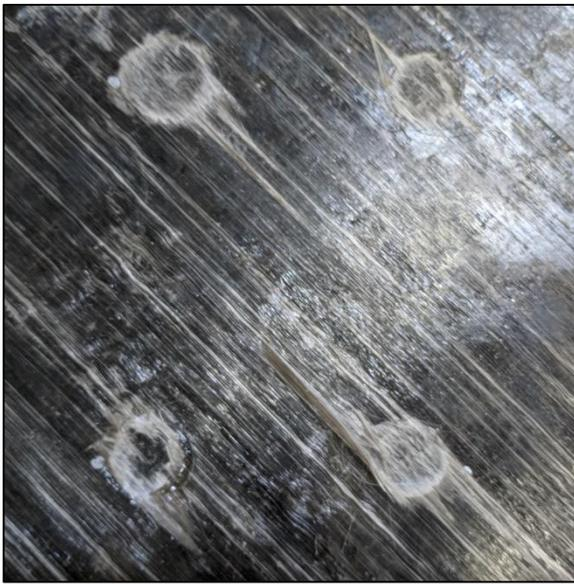
Figure 102: Failed PETg Concrete-TP Stud
