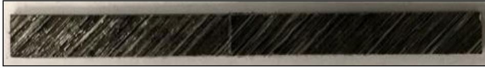
Figure 65: E-glass/PETg [+/- 45 90 0]s Failed Compression Sample
