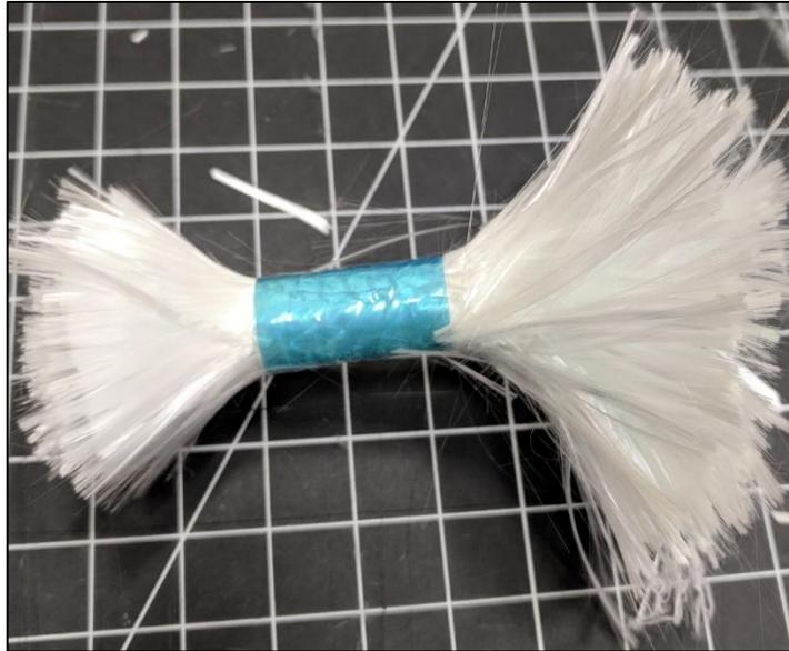
Figure 81: Rolled E-BX 2400 Double Bias E-glass [78] for Infused Stud
