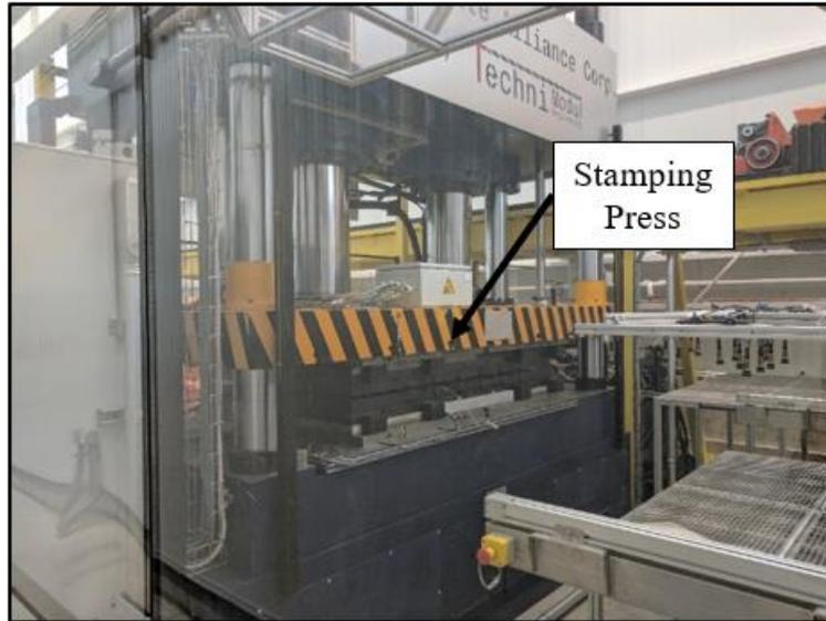
Figure 11: 650 Metric Ton Utah Hydraulic Press
