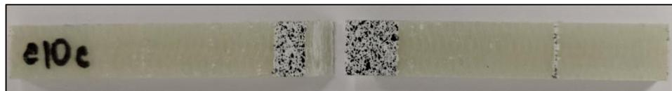
Figure 34: E-glass/Elium UD HAT Failure Trans. Compression Sample
