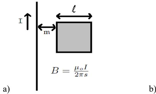
What is the magnetic flux through a square loop (side length  $l$ ), if the first side is a distance  $m$  from the wire?
