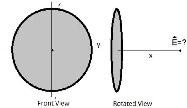
Set up an expression to solve for the electric field a distance,  $x$ , far from the center of the sheet.
