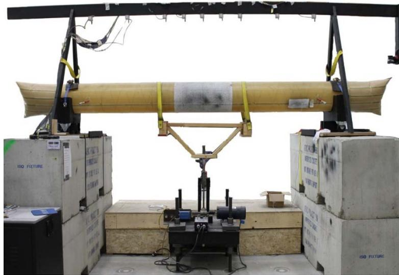
**Figure 4-2. Photo of bending test setup.**
