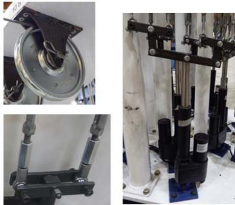
**Figure 5-3. Photo of mechanical improvements implemented by University of Maine: new pulleys and housings (top left), improved cable-to-whiffle tree connections (bottom left), and reduced friction whiffle trees (right).**
