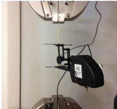
**Figure 3-10. Photo of fiber tow uniaxial tension test specimen with extensometer attached.**
