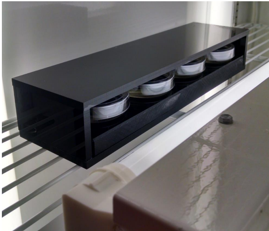
Figure 2.7 Light box used for spore development experiments
