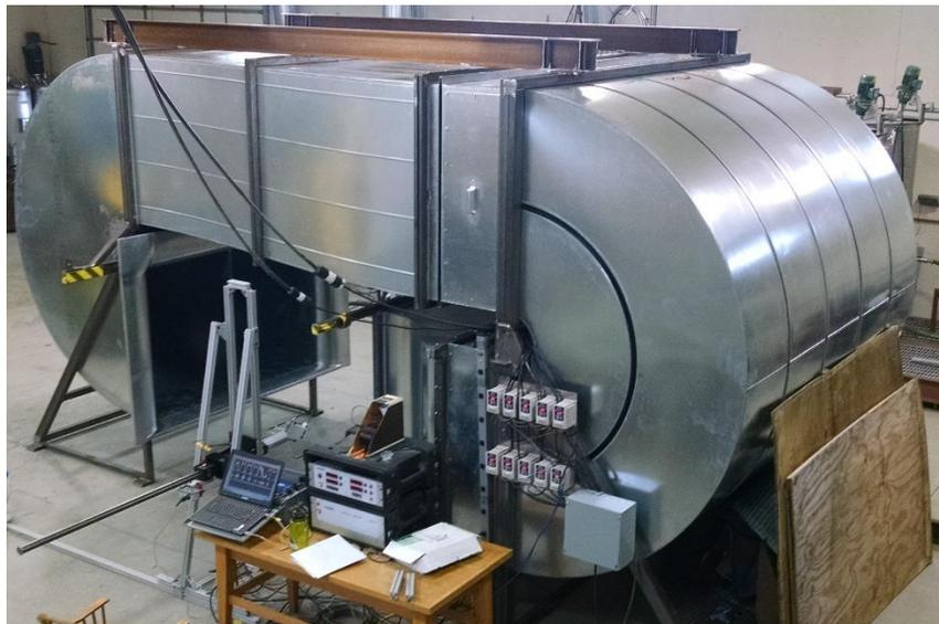
Figure 4.1. Wind tunnel shown in open jet, closed-circuit configuration
