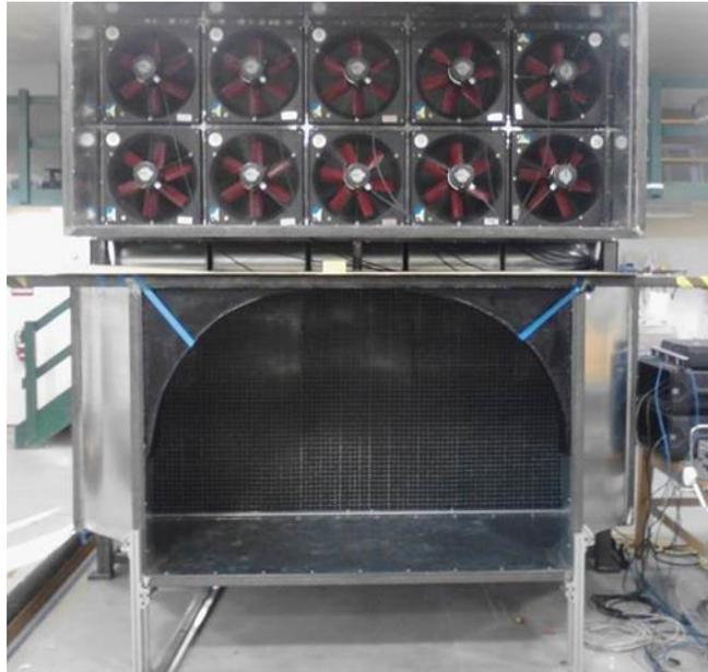
Figure 3.3. The wind generator fan arrangement and nozzle are shown.
