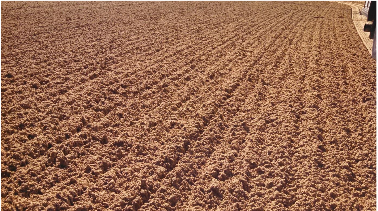
Figure 16: Surface finish of a harrowed track at a typical moisture content.
