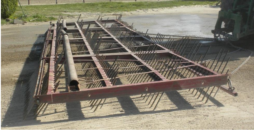
Figure 11: Load controlled harrow showing multiple rows of harrow teeth.
