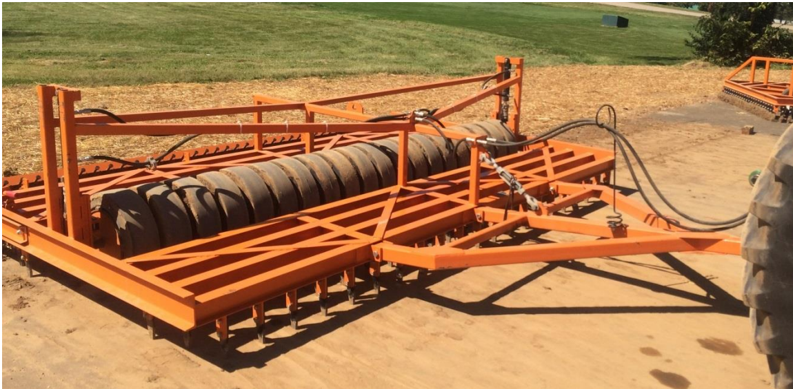
Figure 12: Conditioner with two sets of harrow teeth and the compacting wheels. Some versions of the conditioner are also known as a roller harrow.
