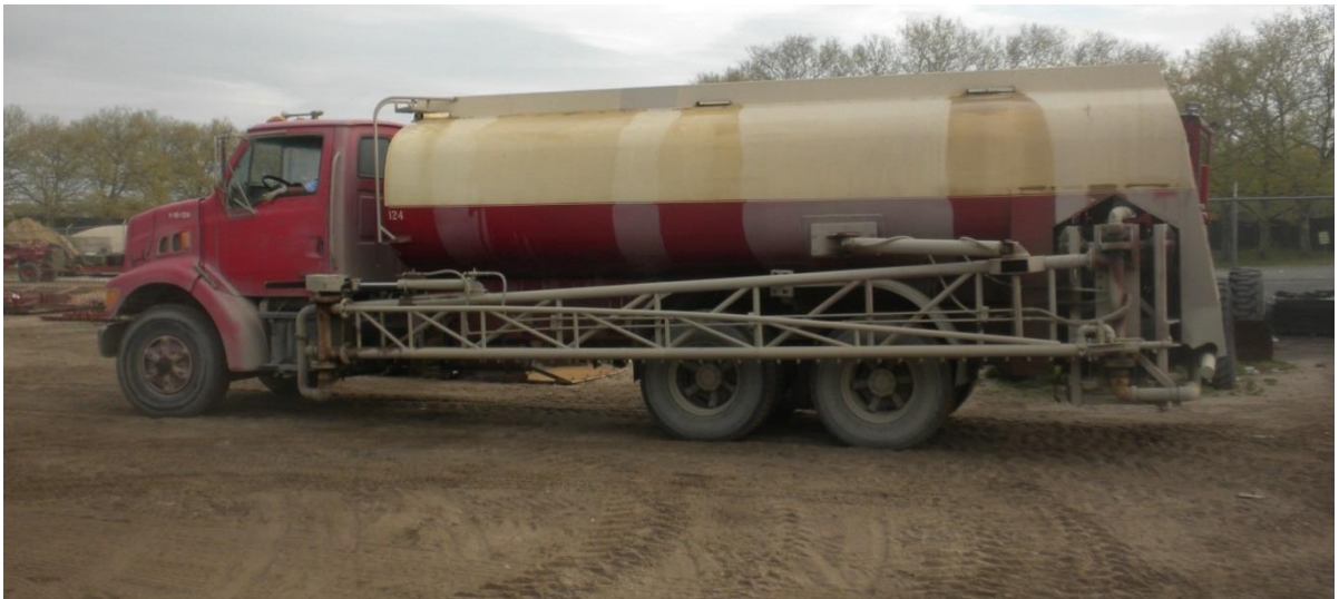
Figure 14: 22.8 m 3 capacity water truck with boom arm retracted.
