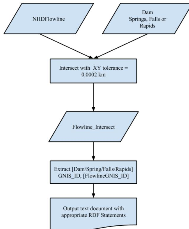
Figure 5.23 Flowchart for Springs, Dam, Falls and Rapids Features
