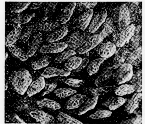
CROSS-SECTION of the new mop yarn. Each cotton fiber strand is jacketed with cellulose sponge material.
