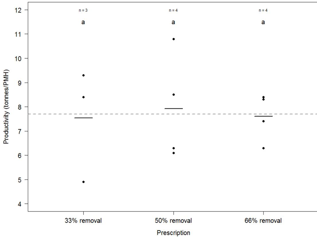
**Figure 3.2:** Harvester productivity in PCT stands for three different treatments. The dashed line represents overall mean productivity, while the solid black lines represent the average productivity for each prescription. Treatments with the same letter are not significantly different from each other.
