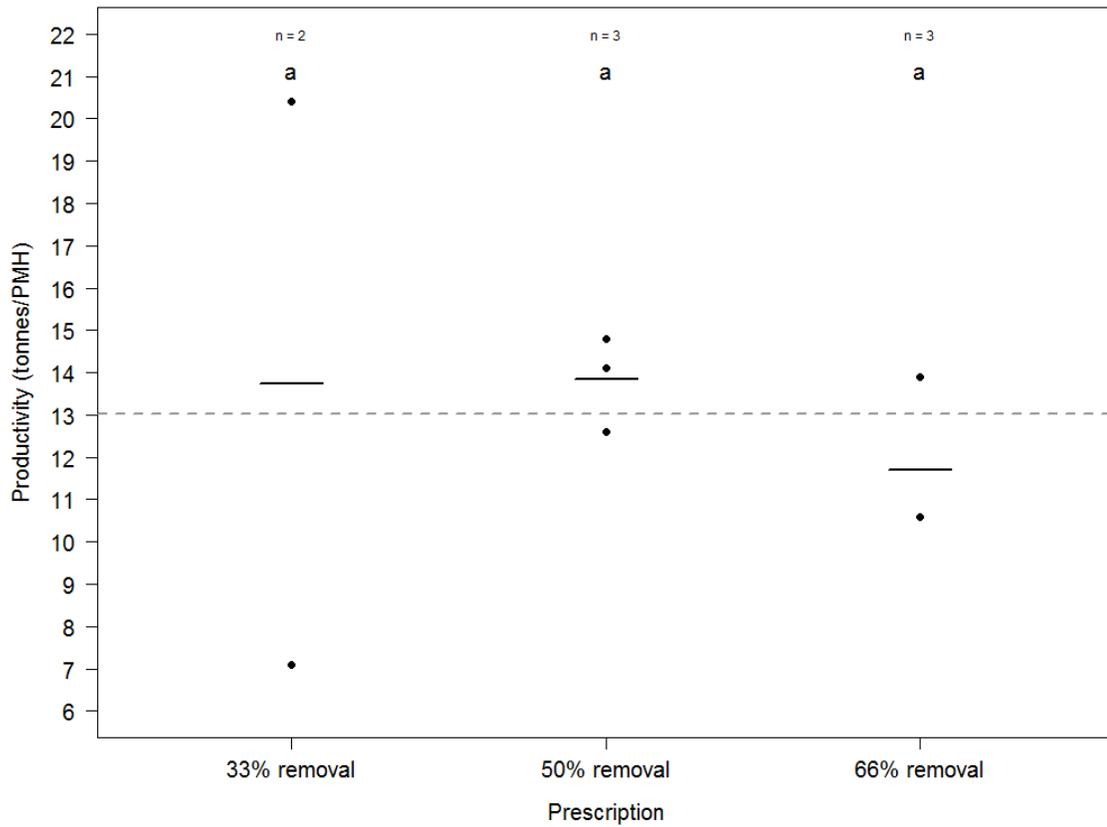
**Figure 3.3:** Feller-buncher productivity in non-PCT stands for three different treatments. The dashed line represents overall mean productivity, while the solid black lines represent the average productivity for each prescription. Treatments with the same letter are not significantly different from each other.
