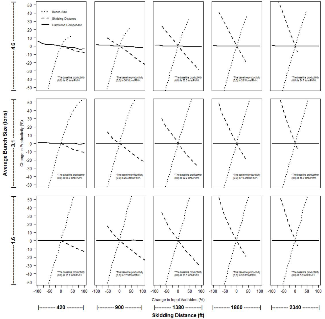
**Figure 1.9:** Global Sensitivity Analysis of three input variables based on baseline conditions consisting of a variety of skidding distances (x-axis), average bunch sizes (y-axis), and a 50% hardwood component.
