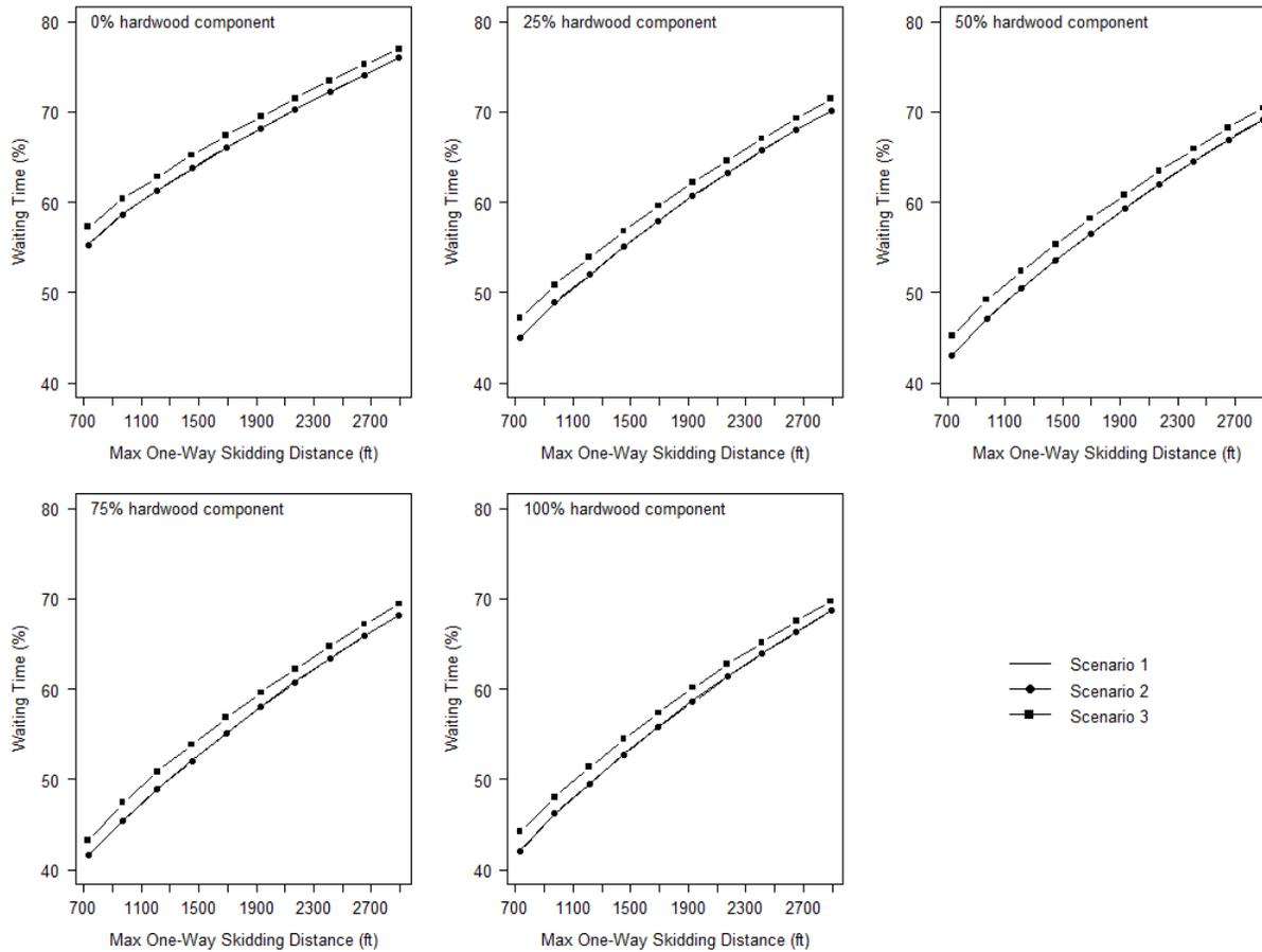
**Figure 1.6:** Stroke delimeter waiting time based on various hardwood components and an average bunch spacing of 48 ft and a removal intensity of 40 tons per acre. No difference was found between Scenario 1 and Scenario 2 and both lines are approximately on top of each other.
