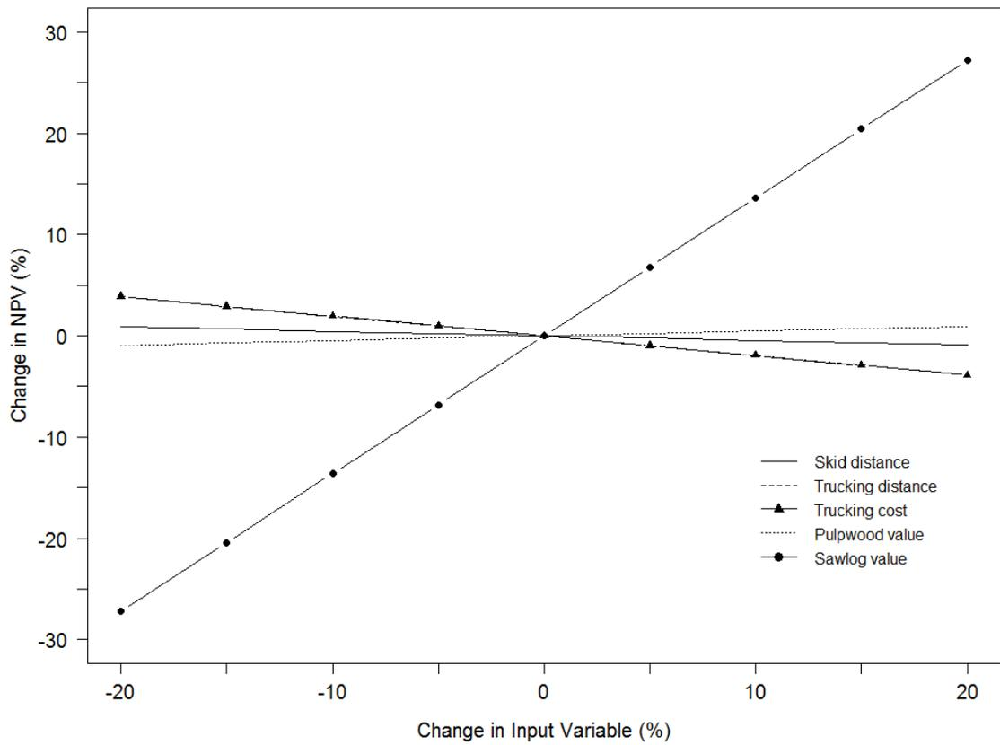
**Figure 4.6:** Sensitivity of net present value to changes in input variables. A change of 0% in input variables represents the baseline conditions as outlined in this manuscript. The curves for a change in trucking distance and trucking costs overlay each other and are not distinct from each other.
