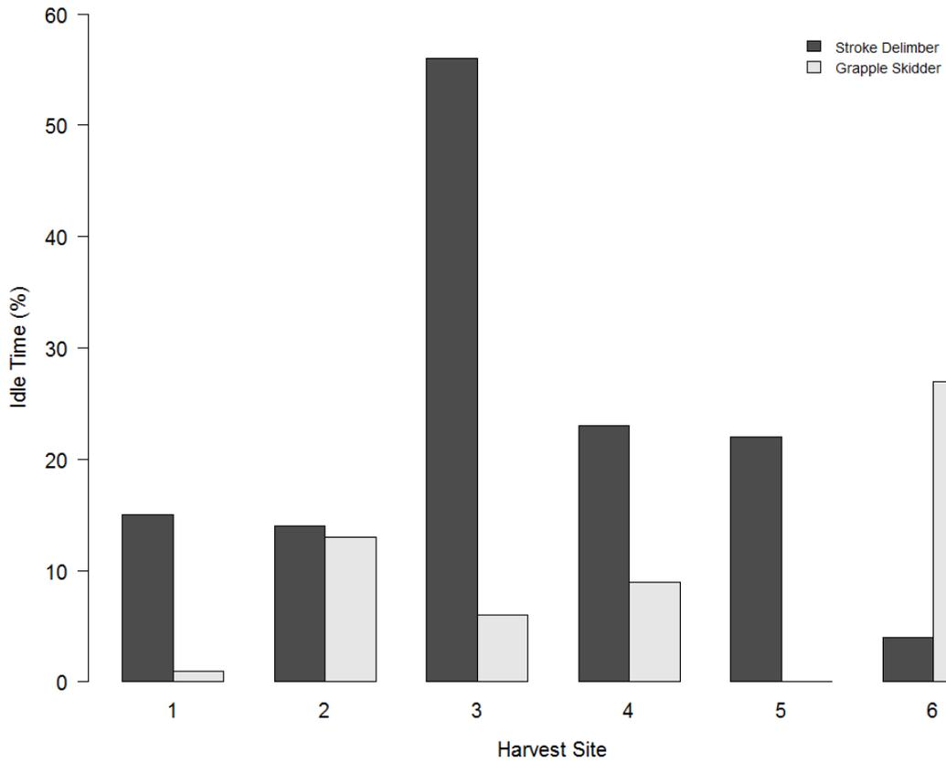
**Figure 1.3:** Observed percent idle time for stroke delimeter and grapple skidder from six different harvest sites as recorded between May and August 2012 by Hiesl (2013). The sites represent a common range of site and stand conditions in Maine.
