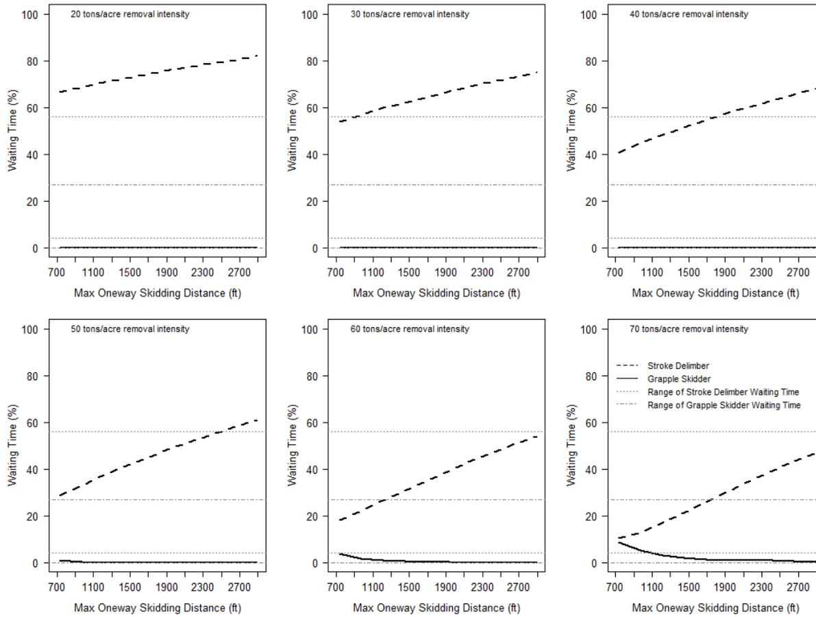
**Figure 1.8:** Waiting time for grapple skidder and stroke delimber based on skidding distance and removal intensity.
