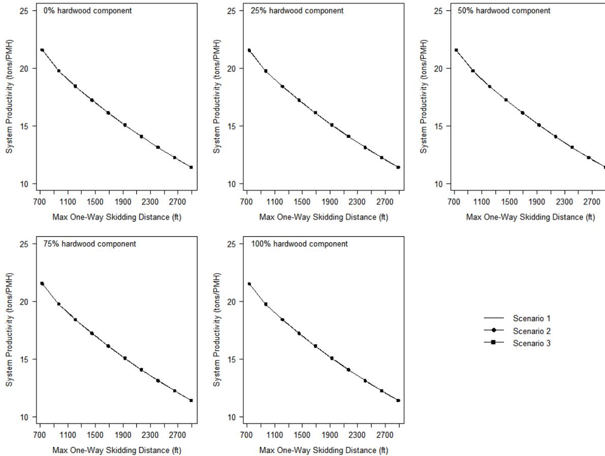
**Figure 1.7:** System productivity of a grapple skidder and stroke delimeter system based on various hardwood components and an average bunch spacing of 48 ft and a removal intensity of 40 tons per acre. The productivity of all three scenarios is similar and thus the individual lines are overlaying each other.
