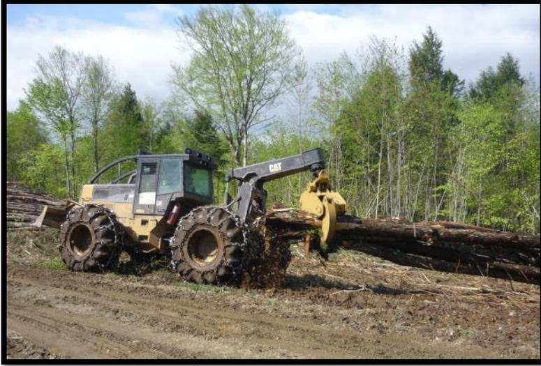
**Figure 1.1:** A grapple skidder generally transports several trees in a bunch from the forest to the roadside where the whole trees get processed by a stroke delimeter.
