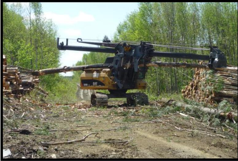
**Figure 1.2:** A stroke delimeter generally processes one tree at a time by cutting of branches and the top above a specific merchantable diameter.
