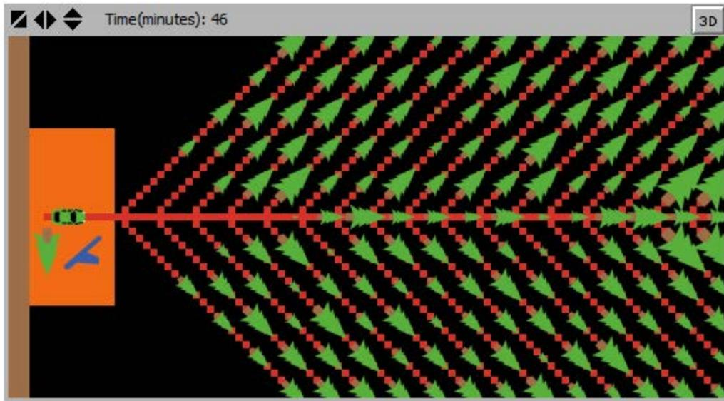
**Figure 2.2:** Screenshot of the trail pattern used in our model, consisting of one main trail and several side trails branching off at a 45 degree angle and a trail spacing of 18.3 m. Individual bunches (green trees on trails) have their butt ends facing towards the extraction route.
