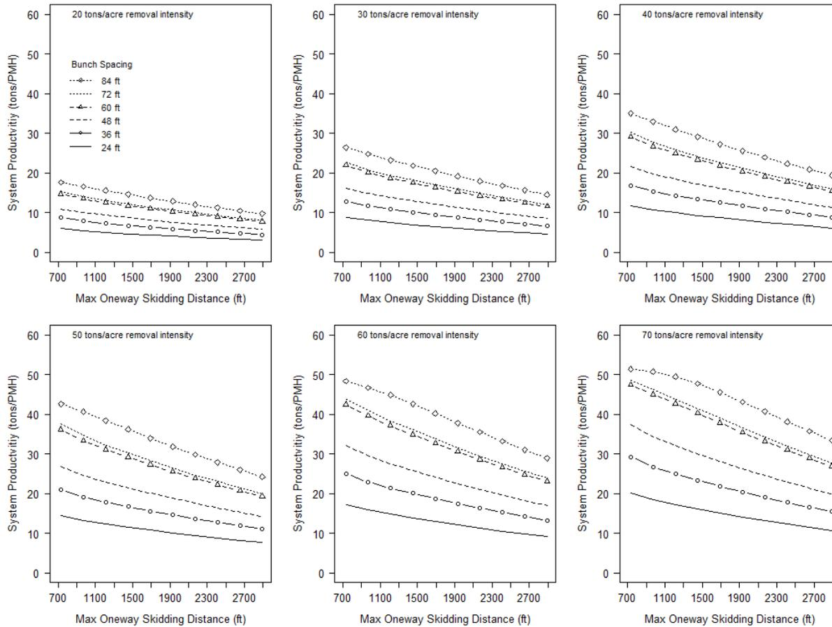
**Figure 1.5:** Grapple skidder and stroke delimeter system productivity based on removal intensity and bunch spacing with a 50% hardwood component when using the baseline scenario (Scenario 1). PMH = productive machine hours.
