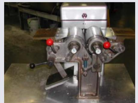
Pictured (top photo) is the laboratory sheet splitter (bottom photo) is the TechPap MorFi Fiber Analyzer.
