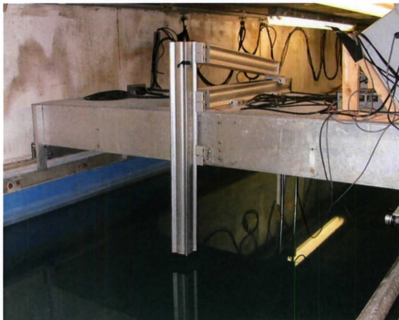
Figure 2.3 – Turbine beam mount on tow tank carriage at the University of Maine tow tank at the Aquaculture Research Center (ARC)
