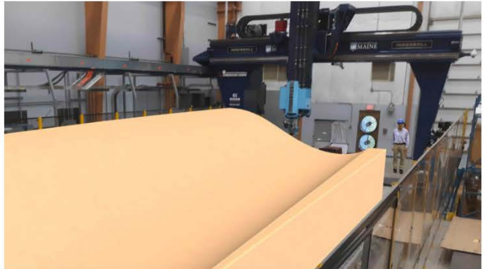
Rendering of a 3D printed wind blade mold segment that will be produced as part of the ASCC's research effort to accelerate wind blade development through additive manufacturing. Researchers will use the world's largest polymer 3D printer to develop recyclable wind blade molds that reduce lead times and costs.
