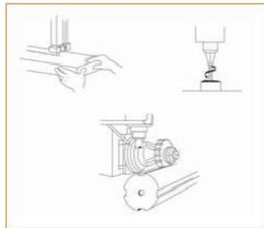
**Cutting Action** occurs by sawing, boring and drilling, milling, and slicing or slitting machinery.
