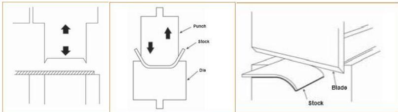
**Punching, Shearing, or Bending Actions** hazard occurs at the point of operation where the worker inserts, holds, or withdraws the stock by hand.
