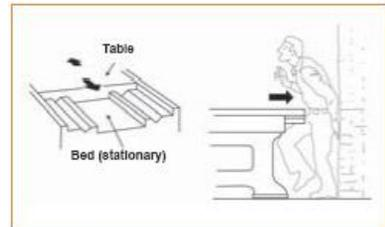
**Reciprocating Motion** is back-and-forth or up-and-down motion that may strike or entrap a worker between a moving part and a fixed object.
