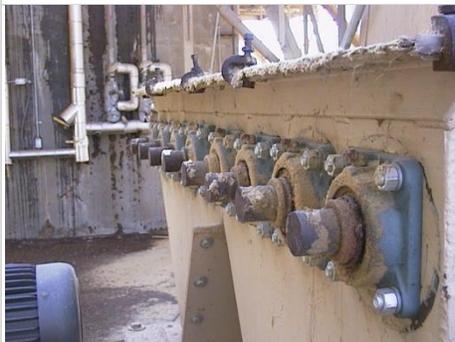
Rotating shaft ends usually project past the bearings. They must be smooth and project less than 1/2 the diameter of the shaft – or they must be guarded.
