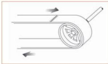
**Transversing Motion** is motion in a straight, continuous line that may strike or catch a worker in a pinch or shear point created by the moving part and a fixed object.
