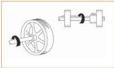
**Rotating Motion** is circular motion such as action generated by rotating collars, couplings, cams, clutches, flywheels, shaft ends, and spindles that may grip clothing or otherwise force a body part into a dangerous location. Projections such as screws or burrs on the rotating part increase the hazard potential.
