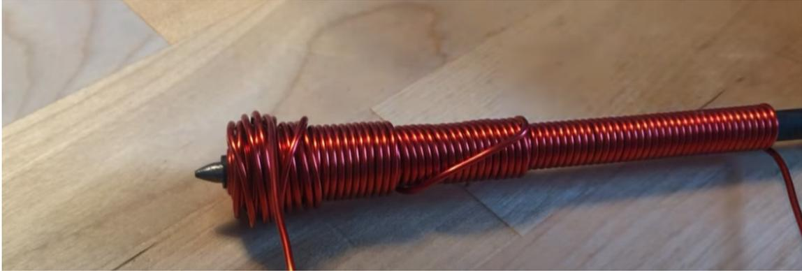
**Figure 22.** Concept of non-cylindrical drive coils for coilguns [17].
