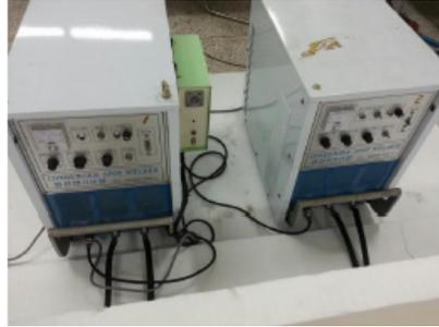
**Figure 6.** Reluctance design power supply (Spot Welders) [11].
