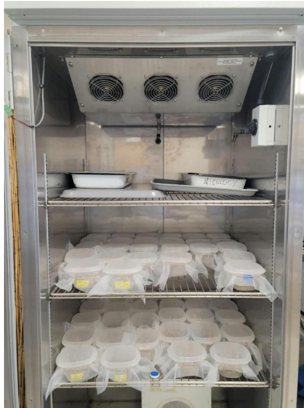
Figure 1. The setup of the 56 container units inside the growth chamber. At the top of the chamber are the pans of water for humidification. The blue Tempo Disc on the bottom shelf recorded temperature and humidity, which was moved to different spots to verify all units experienced consistent conditions.
